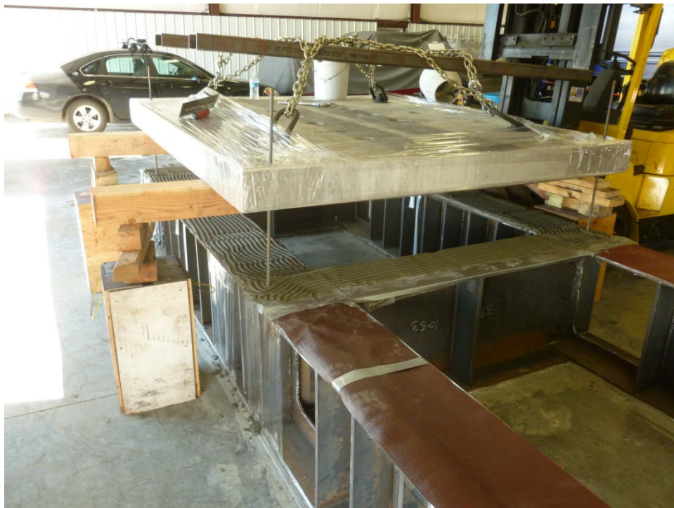
Figure 9: Test panel ready to be set in place on wet grout.
