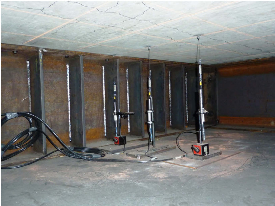
Figure 6: Photo of LVDT sensors attached to underside of a test panel.
