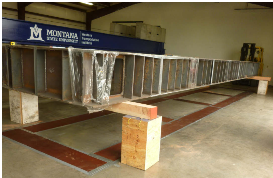
Figure 7: Reaction frame ready to be grouted to the floor.
