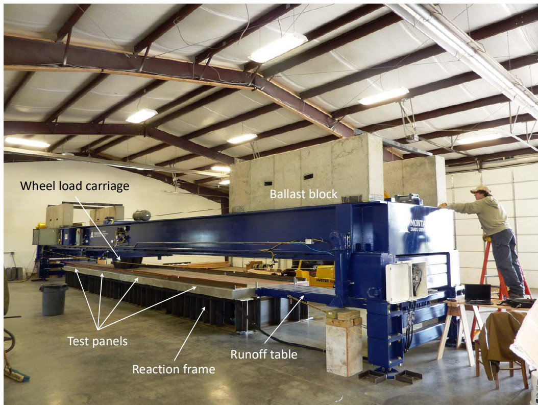
Figure 1: Automated bridge deck tester.
