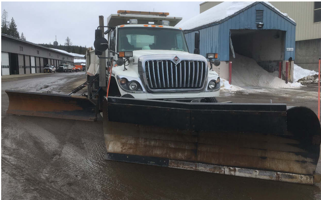
Figure 10: Caltrans 10-Yard Wing Plow with 18-Foot Snow Clearing Path
