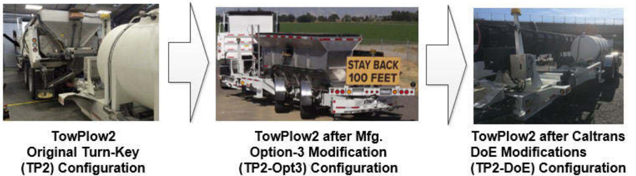
Figure 5: Phases of TowPlow1&2 Configurations
