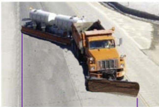
Less Than Two Lanes Clearing with Caltrans 10-ft Head Plow
