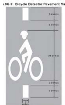
Bicycle Detector Pavement Marking
