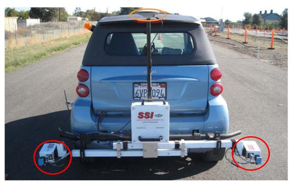
Figure 3.14: SSI lightweight inertial profiler with rear-mounted high-speed lasers in both wheelpaths (red circles) and GPS unit (orange oval).
