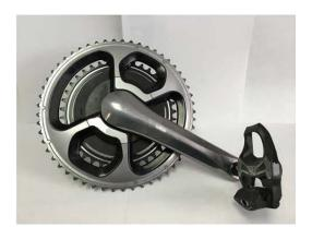
Figure 3.15: Manufacturer A power meter crank, front.
