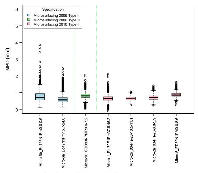
Figure 6.4: Ranges of MPD measured on microsurfacing sections.
