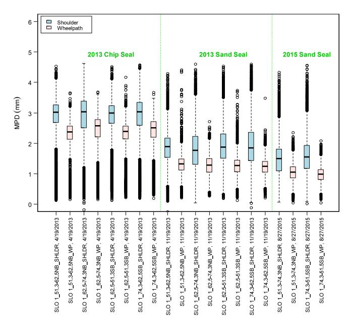
Figure 9.3: MPD over time on the SLO-1 subsections (by post mile and direction) on the shoulder (SHLD) and in the wheelpath (WP).
