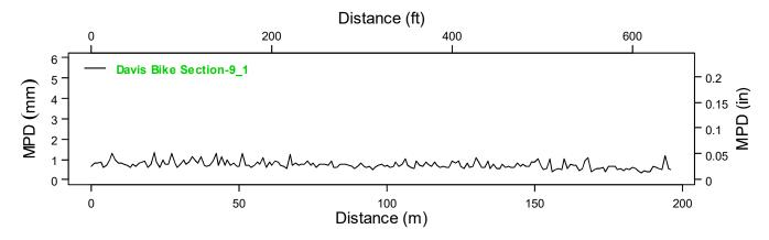
Figure B.3: Macrotexture measured using IP on Davis survey Section 9.
