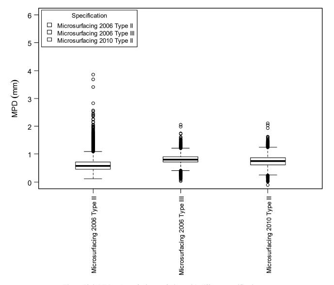
Figure 10.4: MPD values of microsurfacings with different specifications.
