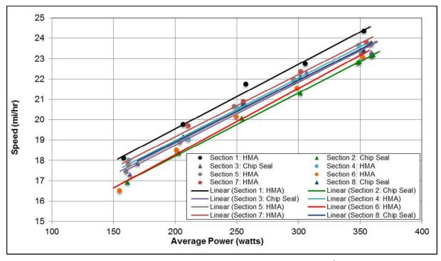
Figure 8.2: Road bicycle power and speed plot of recorded data, given C<sub>D</sub>A=0.383 m<sup>2</sup> and a similar standard road bicycle.
