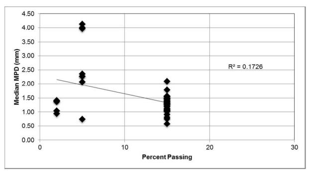
Figure 6.10: Percent passing #4 sieve upper bound versus median MPD for all chip seal sections.
