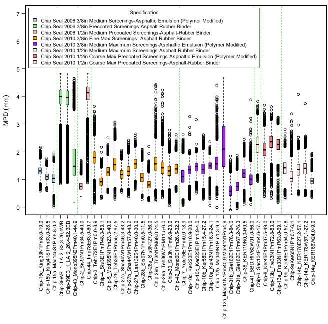
Figure 6.2: Ranges of MPD measured on chip seal sections.
