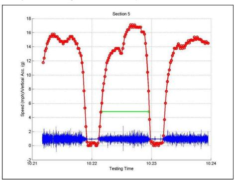
Figure 3.11: Example extract of bicycle speed with corresponding acceleration data. (Note: the red line with circles shows speed (mph), the blue line shows acceleration (g), and the green line shows the test section portion used for analysis where speed > 5 mph.)
