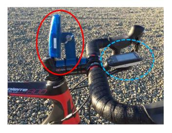
Figure 3.3: Detail of front of road bicycle instrumented with accelerometer (solid red circle) at the stem mounting location and a GPS unit on the handlebar (circle of blue dashes).
