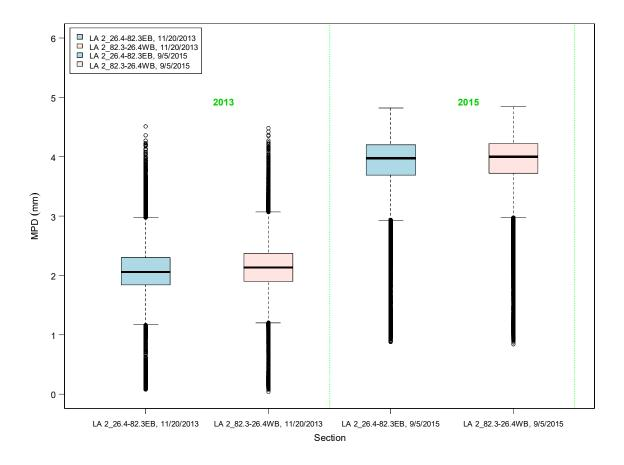
Figure 9.1: MPD over time on LA-2 by direction.
