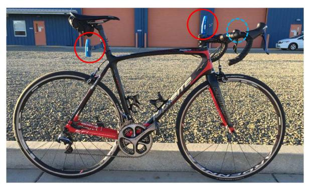
Figure 3.2: Road bicycle instrumented with accelerometers (solid red circles) at the typical mounting locations and a GPS unit on the handlebar (circle of blue dashes).
