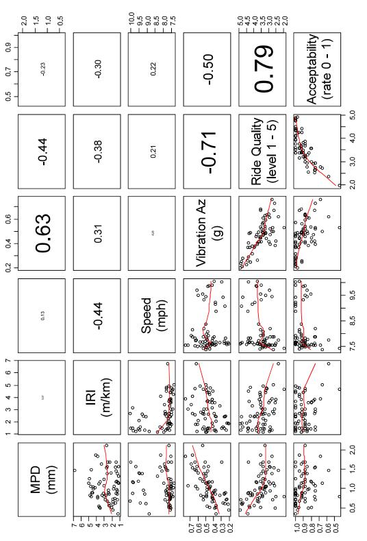
(Note: scatterplots and smooth fitted lines are shown in lower panels. Correlations between variables are shown in upper panels, with the size of the type Figure 4.12: Correlations between MPD, IRI, speed, vibration, ride quality level, and acceptability rate (second study on urban pavements). within the box proportional to absolute correlation.)
