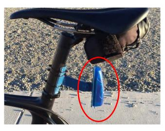
Figure 3.4: Detail of rear of road bicycle instrumented with accelerometer (solid red circle) at the seatpost mounting location.
