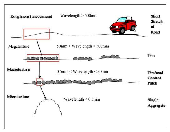
Figure 2.1: Pavement surface texture components and their wavelengths (3). (Note: 500 mm = 1.64 ft, 50 mm = 0.164 ft or 2.0 in., 0.5 mm = 0.02 in.)
