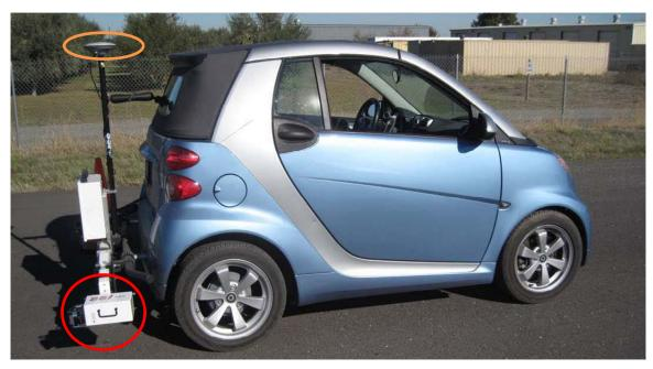
Figure 3.13: SSI lightweight inertial profiler with rear-mounted high-speed lasers, one in each wheelpath (red circle, shows laser in right wheelpath) and GPS unit (orange oval).
