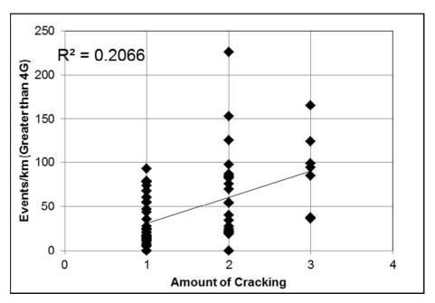
Figure 5.1: Acceleration BQRI (events/km) versus severity of cracking (1 to 3 scale), road bike, rear mount, 4 g event threshold.
