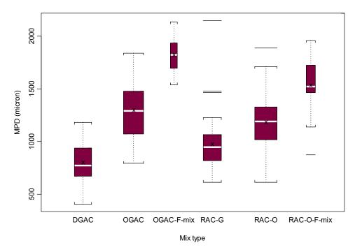
Figure 2.3: Pavement macrotexture (MPD) ranges for different HMA mixture types on California highways considering all ages from new to 16 years of service (7).
