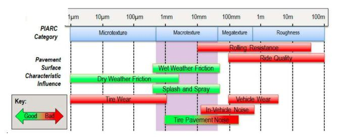
Figure 2.2: Influence of pavement surface texture components on functional performance of motorized vehicles (3).
