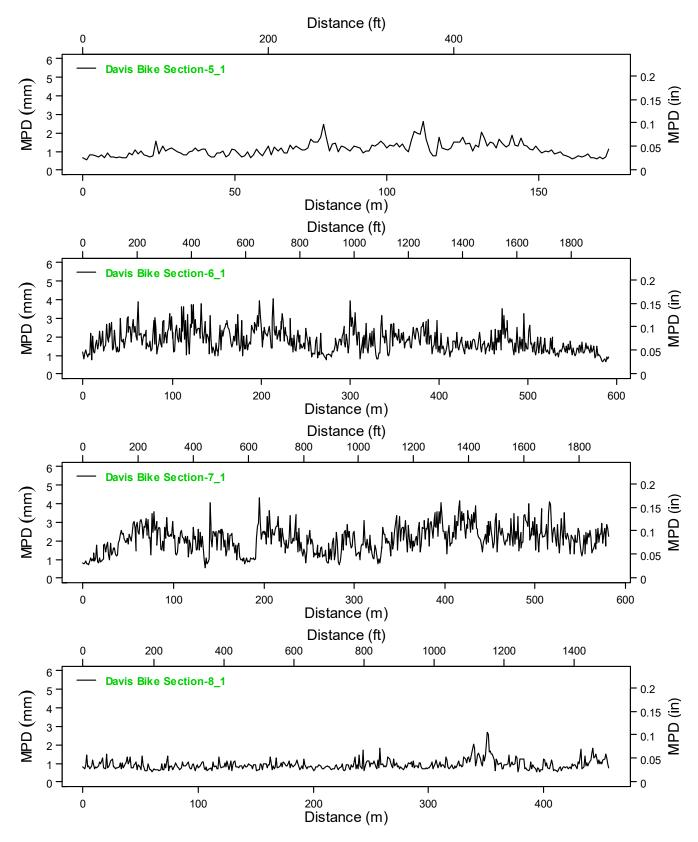
Figure B.2: Macrotexture measured using IP on Davis survey Sections 5 to 8.
