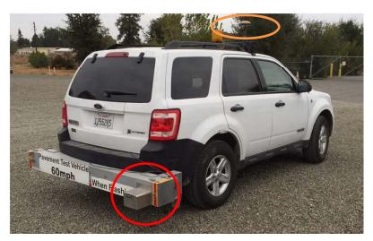
Figure 3.12: UCPRC intertial profiler vehicle with rear-mounted high-speed laser (red circle), in the right wheelpath, and GPS unit (orange oval).
