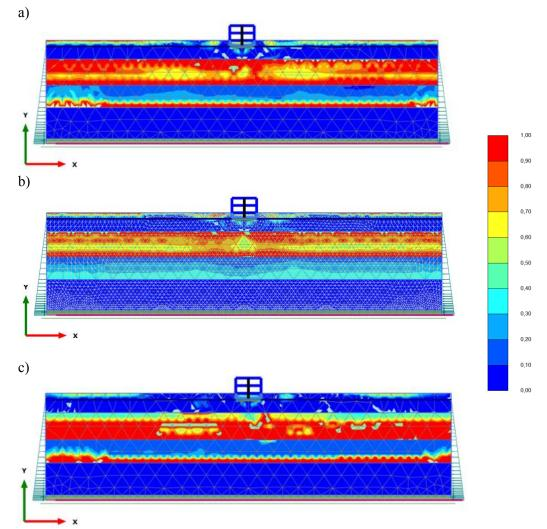
Fig. 74. Pore water pressure ratio ( $r_u$ ) contours for a site supporting a 2-story hypothetical structure when subjected to the CLE conditions: a) Duzce 1999 b) Imperial Valley 1979, and c) Kobe 1995.
