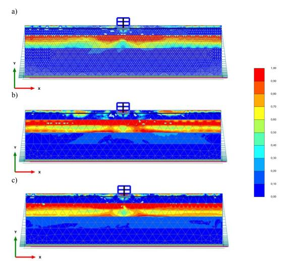
**Fig. 73.** Pore water pressure ratio ( $r_u$ ) contours for a site supporting a 2-story hypothetical structure when subjected to the OLE conditions: a) Whittier 1987, b) Imperial Valley 1979, and c) Superstition Hill 1987.
