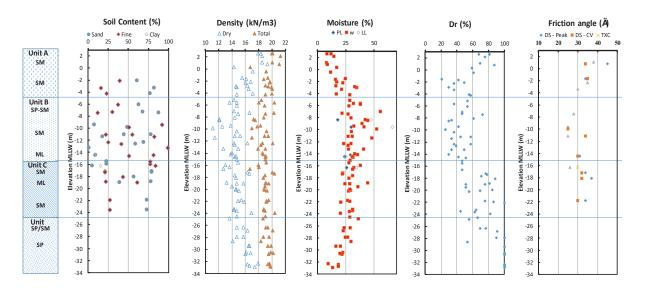
**Fig. 37.** Summary of the geotechnical laboratory testing program for Pier S located within Zone IV (After Geotechnical Professionals Inc. 2003).
