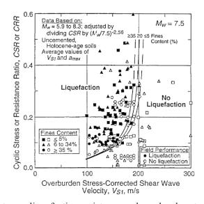
Fig. 12. Relationship between liquefaction resistance and overburden stress-corrected  $V_s$  (Youd et
