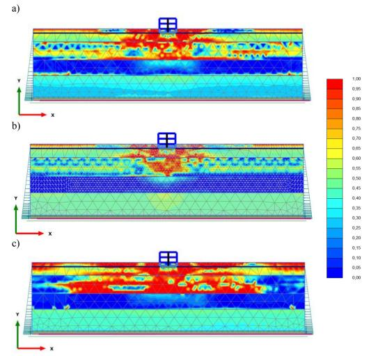
Fig. 76. Relative shear stress ( $\tau_{relative}$ ) contours for a site supporting a 2-story hypothetical structure when subjected to the CLE conditions: a) Duzce 1999 b) Imperial Valley 1979, and c) Kobe 1995.
