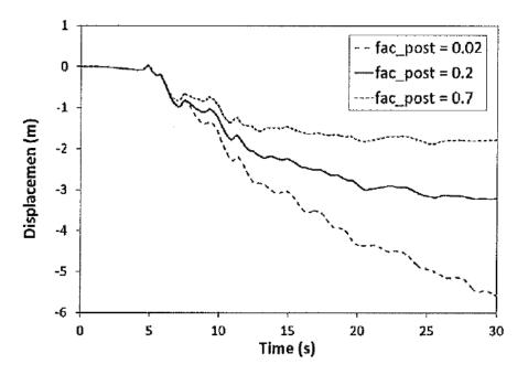
Fig. 21. Effect of *fac<sub>post</sub>* parameter on the computed horizontal displacement in a quay wall in Kobe (Japan) during the Hyogoken-Nambu Earthquake in 1995 (Galavi et al. 2013).
