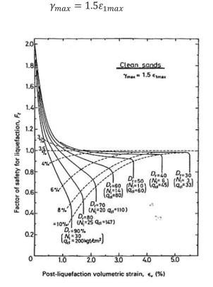
**Fig. 14.** Volumetric strain as a function of  $D_r$ ,  $q_{cl}$ , SPT N-value and FS against liquefaction (after Ishihara and Yoshimine 1992).
