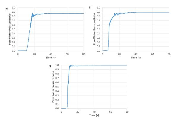
Fig. 58. Pore pressure ratio ( $r_u$ ) through the dynamic time for the Unit B for the CLE conditions a) Duzce 1999, b) Imperial Valley 1979 and c) Kobe 1995.
