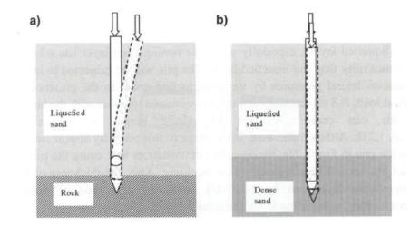
Fig. 17. Collapse modes for individual piles founded in: a) rock, b) compact sandy soils (Madabhushi et al. 2010).
