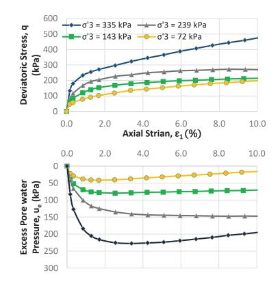
Fig. 49. CIU-TXC tests conducted by AP Engineering and Testing, Inc. at the project site.
