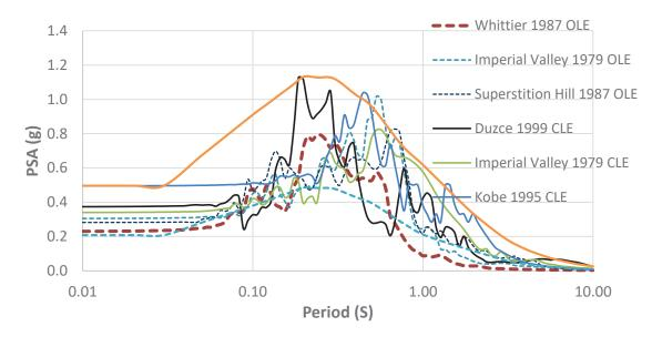
Fig. 69. Acceleration response spectra at the top of the ground surface with DEEPSOIL for the OLE and CLE conditions.
