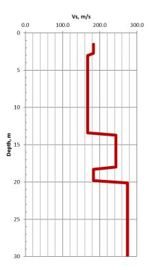
Fig. 34. Results of shear wave velocities for Pier S located within Zone IV (After Earth Mechanics Inc. 2006).
