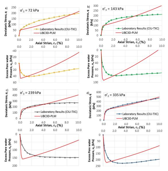
Fig. 50. Comparison of CIU-TXC test results and numerical simulations using UBC3D-PLM model in PLAXIS 2D for different confining pressures: a) σ'<sub>c</sub>=72 kPa, b) σ'<sub>c</sub>=143 kPa, c) σ'<sub>c</sub>=239 kPa and d) σ'<sub>c</sub>=335 kPa.
