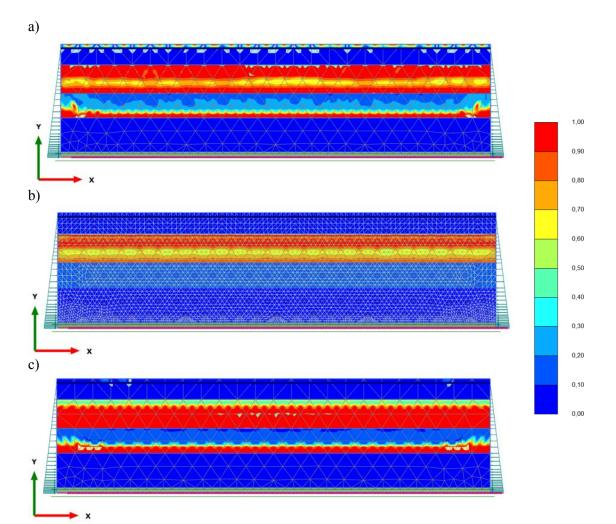
Fig. 56. Pore water pressure ratio  $(r_u)$  contours for the CLE condition a) Duzce 1999 b) Imperial Valley 1979 and c) Kobe 1995.
