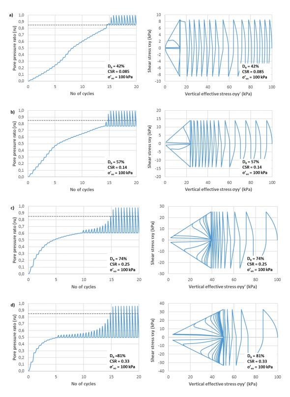
Fig. 46. Results of pore pressure ratios and stress paths computed from the numerical simulations of undrained cyclic direct simple shear tests obtained with the numerical model for different  $D_r$  values a) 42%, b) 57%, c) 74% and d) 81%.
