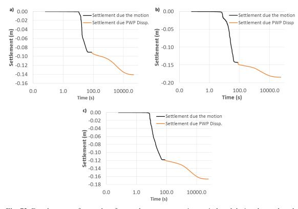
Fig. 72. Development of ground surface settlements versus time as induced during the earthquake and during the pore water pressure dissipation phase for CLE condition: a) Duzce 1999 b) Imperial Valley 1979, and c) Kobe 1995.
