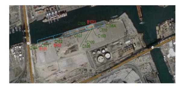
**Fig. 35.** Approximate location of CPT and SPT soundings (After Geotechnical Professionals Inc. 2003).
