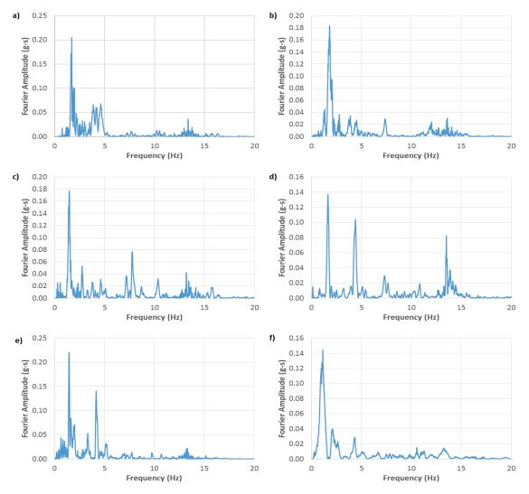
**Fig. 66.** Fast Fourier amplitude at the top ground surface with PLAXIS 2D for the OLE condition a) Whittier 1987, b) Imperial Valley 1979, c) Superstition Hill 1987 and CLE condition d) Duzce 1999 e) Imperial Valley 1979 and f) Kobe 1995.
