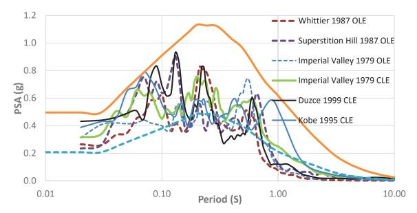
**Fig. 68.** Acceleration response spectra at the top of the ground surface with PLAXIS 2D for the OLE and CLE conditions.
