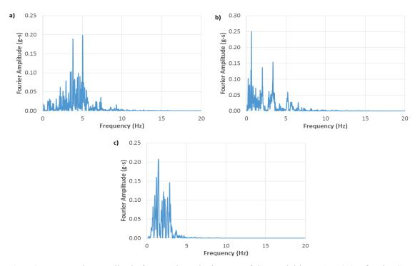
**Fig. 54.** Fast Fourier amplitude for a node at the bottom of the model in PLAXIS 2D for the CLE condition: a) Duzce, b) Imperial Valley, and c) Kobe.
