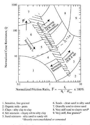
Fig. 11. CPT-Based soil behavior-type chart (after Robertson and Wride 1998).
