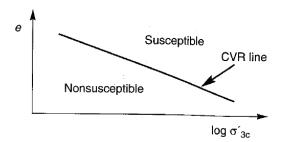
**Fig. 6.** *CVR* as a boundary of contractive and dilative states to assess liquefaction susceptibility (Kramer 1996).
