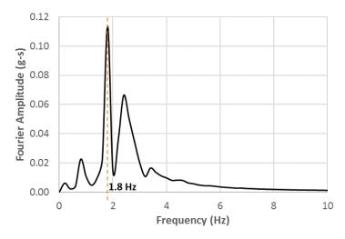
Fig. 70. Fast Fourier amplitude for the 2-story structure with a basement level using PLAXIS 2D.
