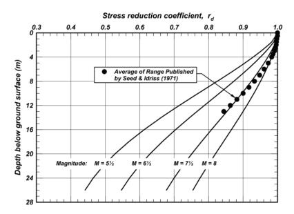
Fig. 7. Shear stress reduction factor relationship (Idriss and Boulanger 2010).
