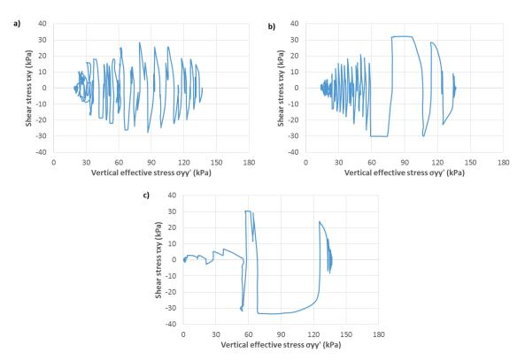
**Fig. 64.** Stress path for a point in the middle of Unit B for the CLE condition: a) Duzce 1999 b) Imperial Valley 1979 and c) Kobe 1995.
