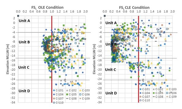
**Fig. 42.** Factor of safety to evaluate liquefaction susceptibility using CPT semi-empirical method for the OLE and CLE condition.
