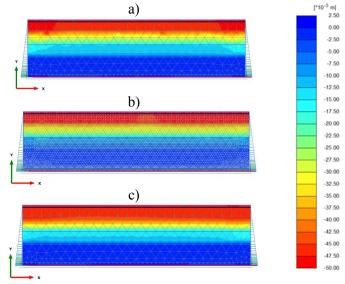
**Fig. 60.** Maximum vertical deformation contours for the OLE condition after the pore water pressure dissipation a) Whittier 1987, b) Imperial Valley 1979, and c) Superstition Hill 1987.
