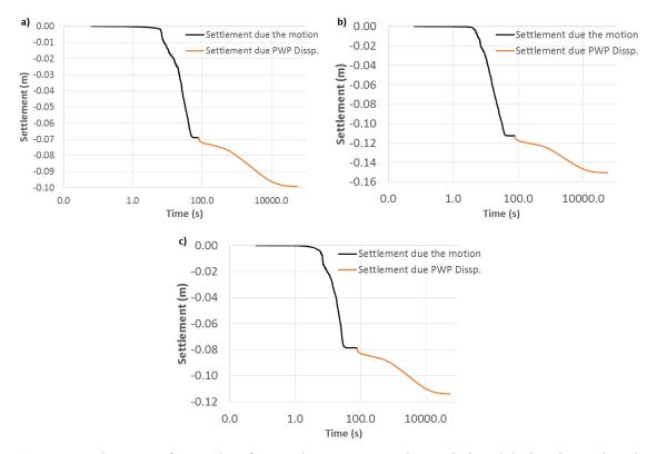
Fig. 71. Development of ground surface settlements versus time as induced during the earthquake and during the pore water pressure dissipation phase for OLE condition: a) Whittier 1987,b) Imperial Valley 1979, and c) Superstition Hill 1987.
