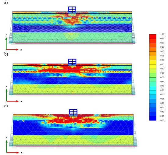
Fig. 75. Relative shear stress ( $\tau_{relative}$ ) contours for a site supporting a 2-story hypothetical structure when subjected to the OLE conditions: a) Whittier 1987, b) Imperial Valley 1979, and c) Superstition Hill 1987.
