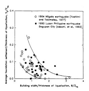
**Fig. 16**. Normalized foundation settlements versus normalized building width for the 1964 Niigata (Japan) and 1990 Luzon (Philippines) earthquakes (Liu and Dobry 1997).
