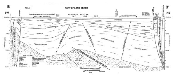
Fig. 29. Geological cross section B-B' of POLB area (Earth Mechanics Inc. 2006).
