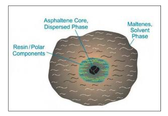
Figure 2.1: Asphalt binder colloidal structure (9).
