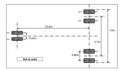
Figure 10.25: Boeing 737-800 gear footprint.
