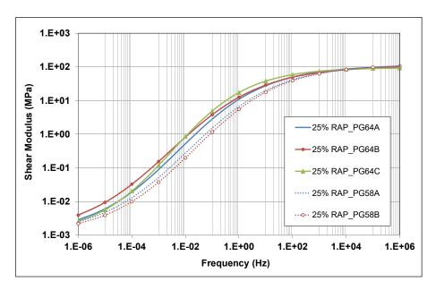
Figure 7.7: Shear moduli of binders with 25 percent RAP binder replacement (20°C).
