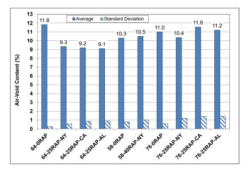
Figure 9.4: Air-void content of FAM mixes.
