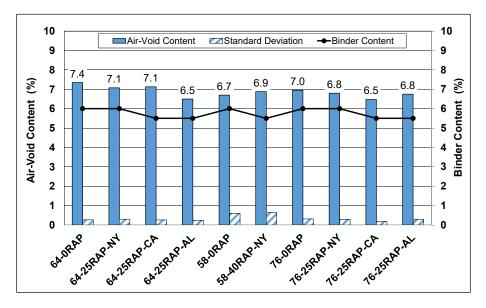
Figure 10.15: Average air-void contents of Hamburg Wheel-Track Test specimens.
