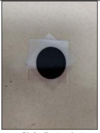
b. Making binder disc using DSR
