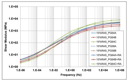
Figure 7.18: Master curves of FAM mixes with 15 percent RAS binder replacement.
