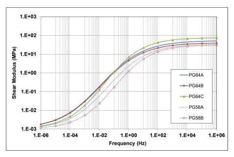
Figure 7.6: Shear moduli of virgin asphalt binders (20°C).
