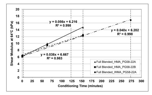
Figure 5.8: Aging coefficient for HMA and WMA production paths.
