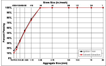
Figure 8.18: Fine aggregate gradation of New York RAP.
