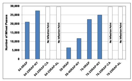
Figure 10.19: Approximate Hamburg Wheel-Track Test inflection points.
