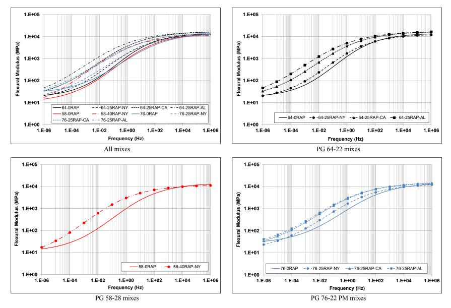
Figure 10.7: Flexural modulus master curves for full-graded mixes.
