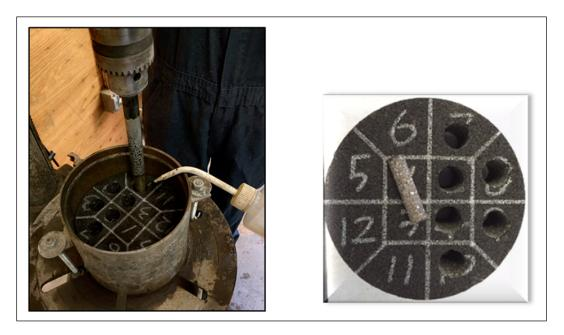
Figure 7.1: FAM mix specimens cored from a Superpave gyratory-compacted specimen.
