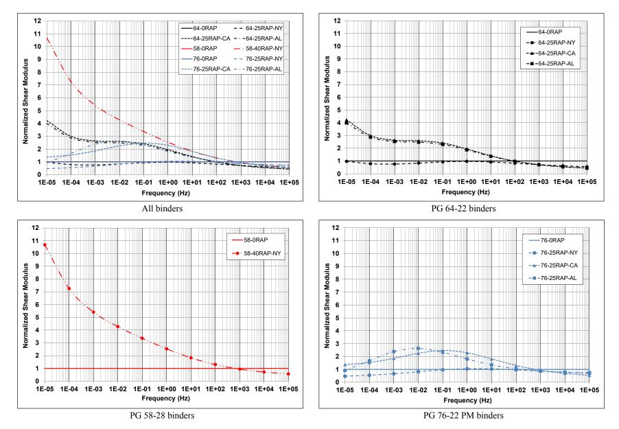
Figure 9.3: Normalized shear moduli master curves for asphalt binders (20°C).
