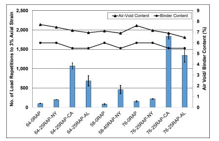
Figure 10.10: Average number of load repetitions to reach 3% axial strain at 52°C.
