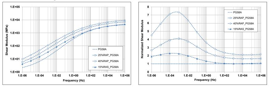
Figure 7.20: PG 58-22-A: Shear and normalized modulus master curves of FAM mixes.
