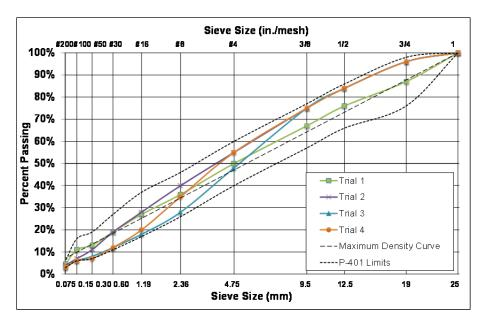
Figure 8.8: Gradation curves for trial aggregate structures.
