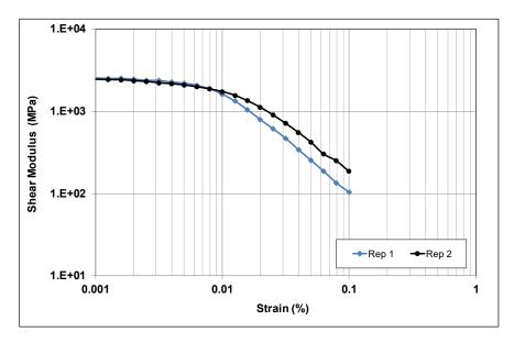
Figure 7.3: Example FAM mix specimen amplitude sweep test results.
