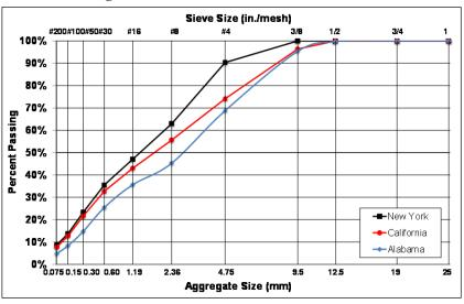
Figure 8.4: Comparison of RAP aggregate gradations by solvent extraction.
