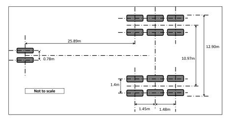
Figure 10.26: Boeing 777F gear footprint.
