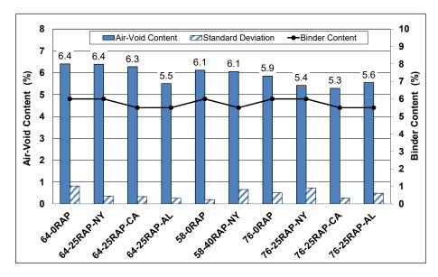
Figure 10.20: Average air-void contents of beam fatigue test specimens.
