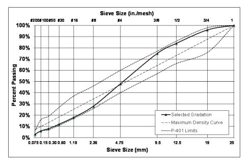
Figure 8.9: Gradation curve for selected aggregate structure.
