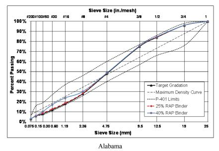
Figure 8.12: Aggregate gradations of mixes with 25 and 40 percent RAP.
