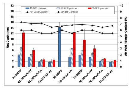
Figure 10.17: Average Hamburg Wheel-Track Test rut depth.
