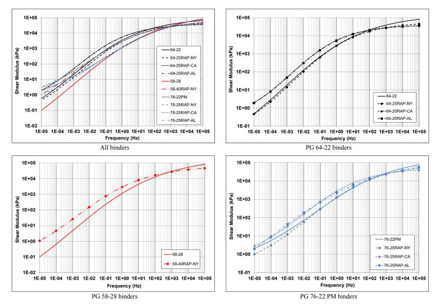
Figure 9.2: Shear moduli master curves for asphalt binders (20°C).
