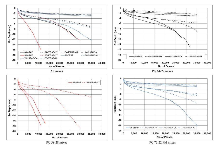
Figure 10.16: Average Hamburg Wheel-Track Test rut progression for full-graded mixes.
