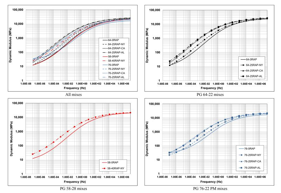
Figure 10.2: Dynamic shear modulus master curves for full-graded mixes.
