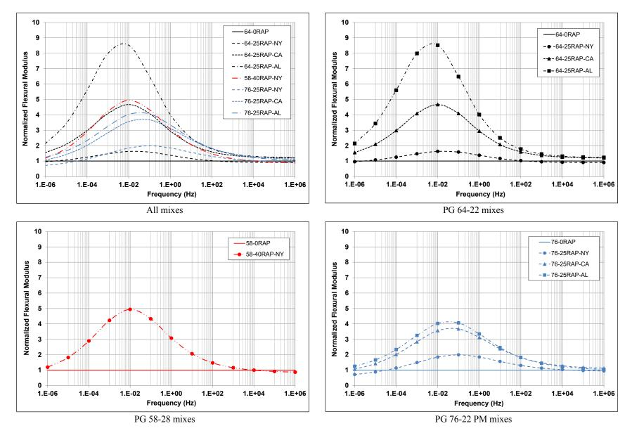
Figure 10.8: Normalized flexural modulus master curves for full-graded mixes.
