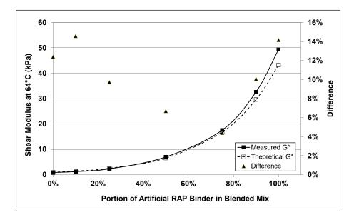
Figure 5.7: Comparison of measured and predicted shear modulus using the Arrhenius rule.
