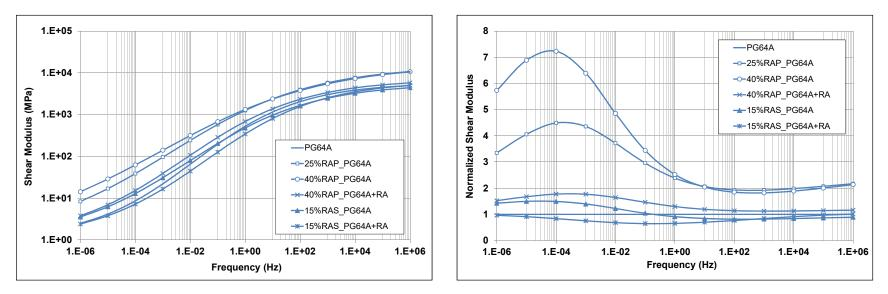
Figure 7.19: PG 64-16-A: Shear and normalized modulus master curves of FAM mixes.
