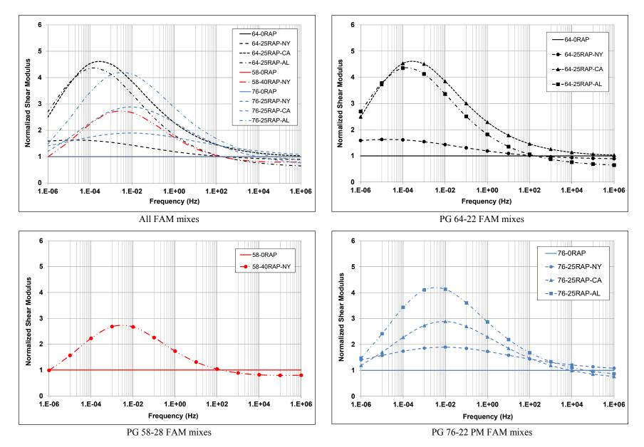
Figure 9.6: Normalized shear moduli master curves for FAM mixes (20°C).
