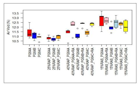
Figure 7.11: FAM mix specimen air-void contents for PG 64 mixes.
