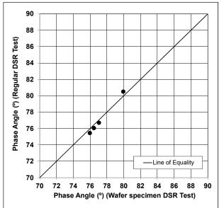
Figure 5.3: Phase angle (δ) test results for fully blended wafer binder specimen.
