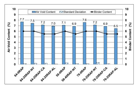
Figure 10.1: Average air-void contents of dynamic modulus specimens.
