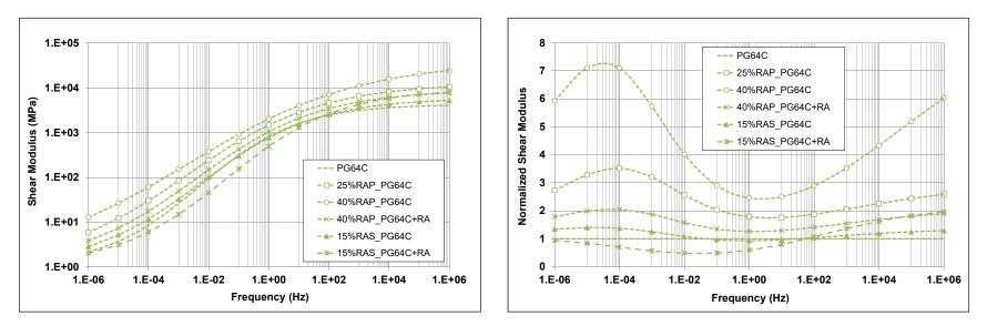
Figure 7.23: PG 64-16-C: Shear and normalized modulus master curves of FAM mixes.
