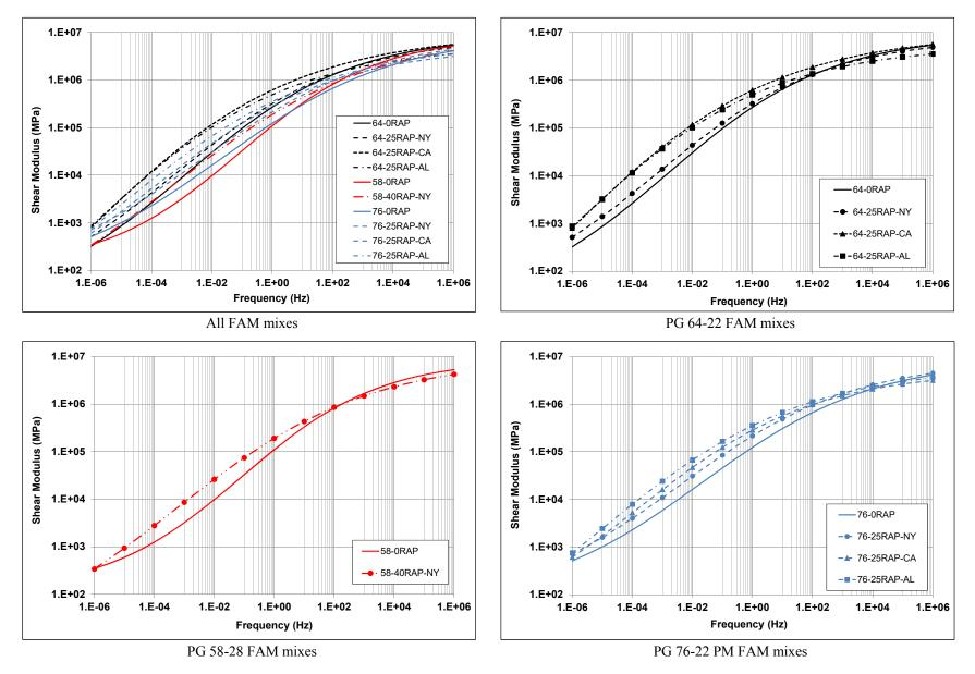
Figure 9.5: Shear moduli master curves for FAM mixes (20°C).
