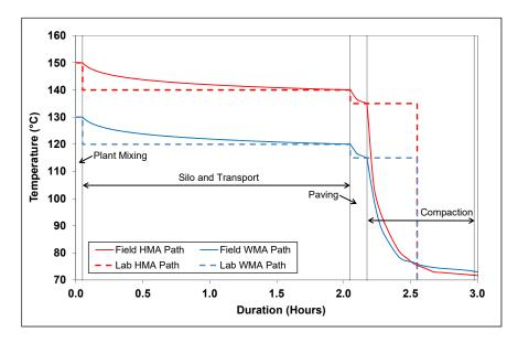
Figure 5.4: Example time-temperature profiles for HMA and WMA from mixing through compaction.
