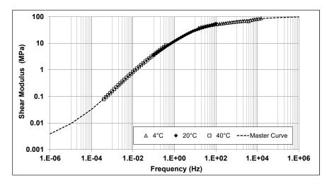
Figure 4.2: Example of a developed master curve for an asphalt binder at 20°C.
