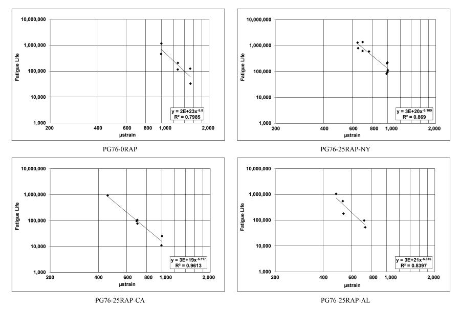
Figure 10.23: Fatigue models for PG 76-22 PM mixes.
