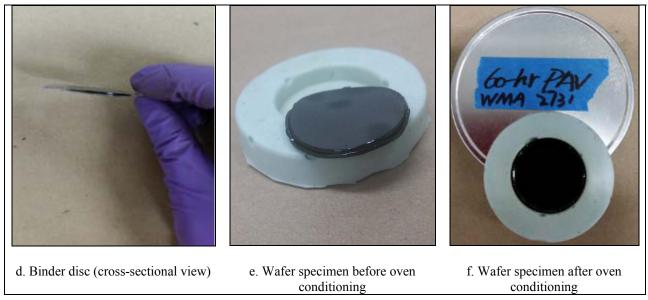
Figure 5.1: DSR contact-blending test sample preparation procedure (continued).
