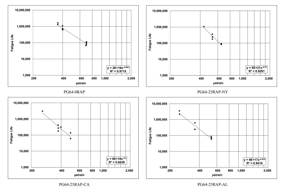
Figure 10.21: Fatigue models for PG 64-22 mixes.
