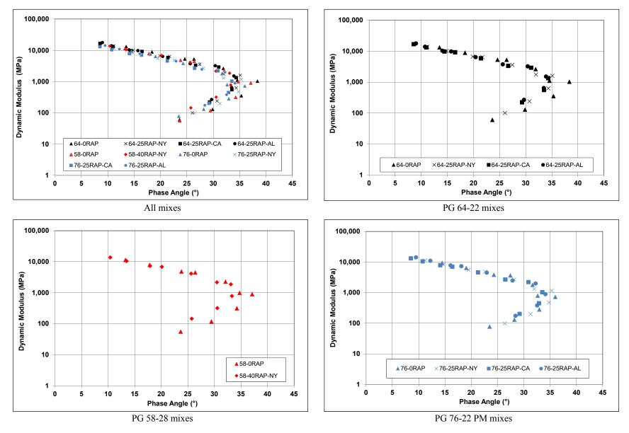
Figure 10.5: Phase angle Black diagrams for full-graded mixes.
