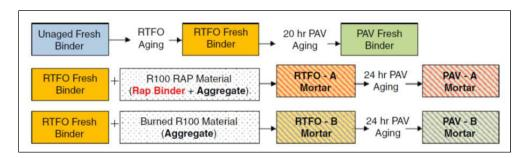
Figure 6.1: Sample preparation for asphalt mortar testing (After Hajj et al. [11]).
