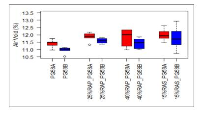
Figure 7.12: FAM mix specimen air-void contents for PG 58 mixes.
