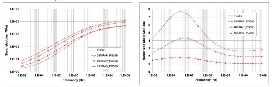
Figure 7.22: PG 58-22-B: Shear and normalized modulus master curves of FAM mixes.
