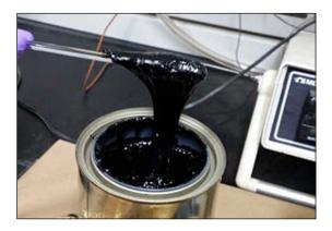
Figure 4.3: Recovered RAS binder after three hours of conditioning at 190°C.
