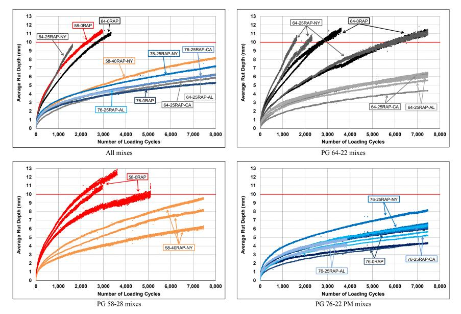
Figure 10.14: Average Asphalt Pavement Analyzer rut progression for full-graded mixes.
