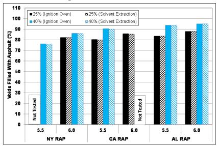
Figure 8.15: Voids filled with asphalt.
