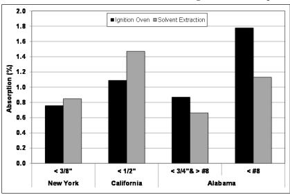
Figure 8.7: Absorption of RAP aggregate.
