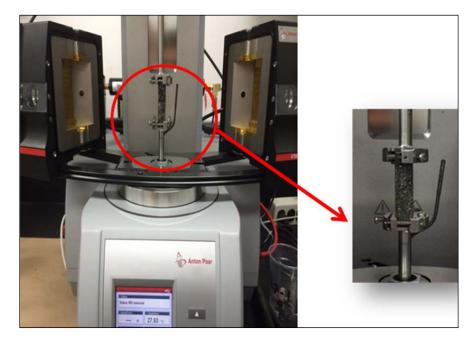
Figure 7.2: DSR-DMA torsion bar fixture used for FAM mix testing.
