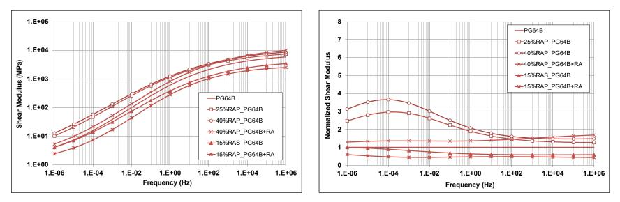
Figure 7.21: PG 64-16-B: Shear and normalized modulus master curves of FAM mixes.
