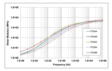
Figure 7.15: Master curves of control FAM mixes.
