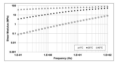
Figure 4.1: Example of measured shear modulus of an asphalt binder at 20°C.
