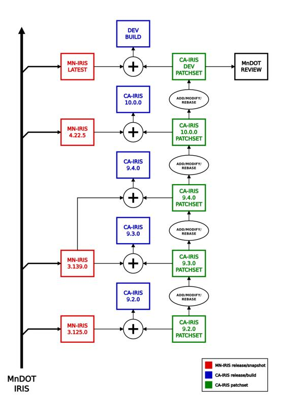
Figure 2.6: Caltrans IRIS source code management workflow
