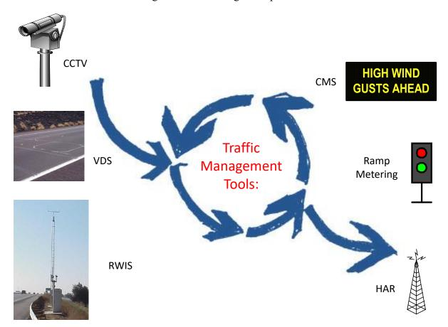
Figure 2.1: ATMS real-time functions
