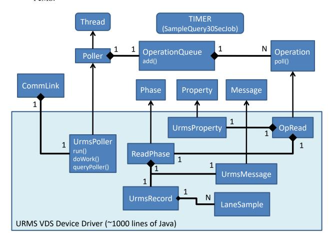
Figure 3.16: IRIS class structure for URMS device driver
