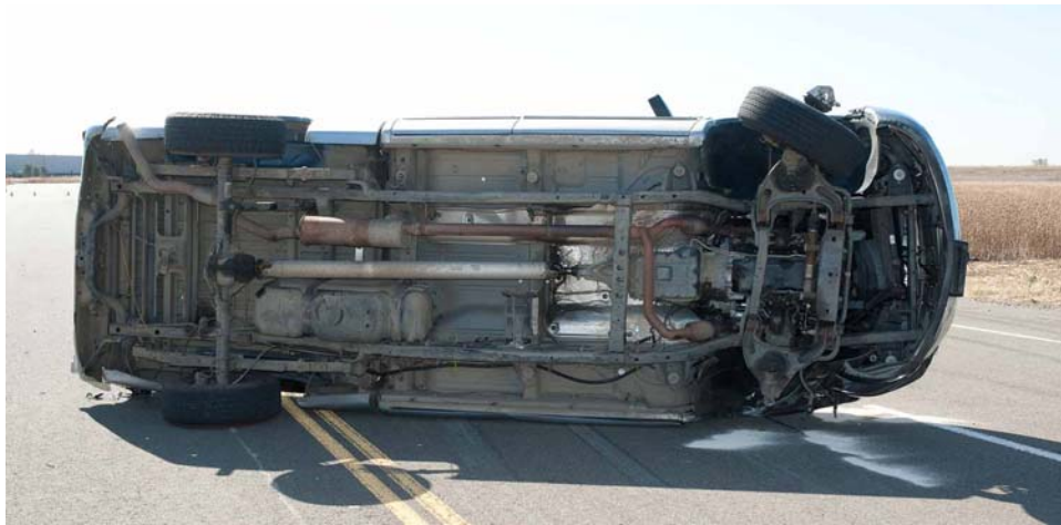
Figure 5-13 Bottom of Vehicle on Its Side After Test 130MASH3P13-03
