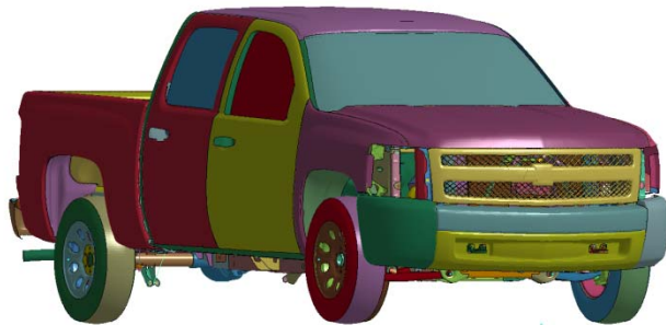
Figure 10-17 MASH 2270P Test Vehicle
