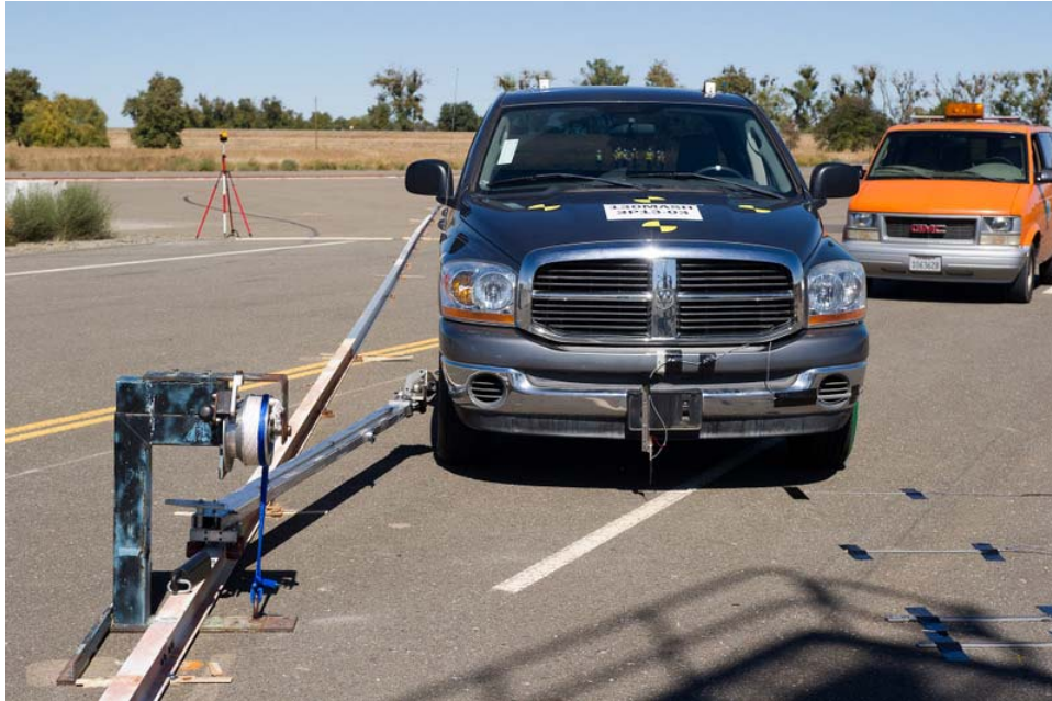
Figure 4-2 Guidance Arm Release Mechanism
