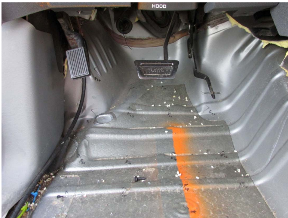
Figure 5-19 Vehicle Floorboard Post Test
