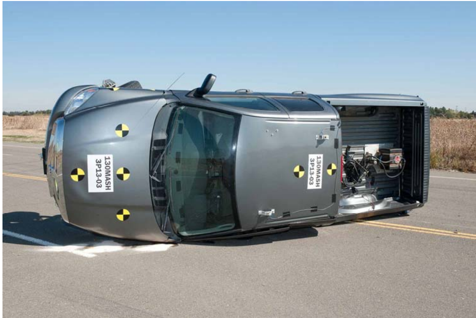
Figure 5-11 Top of Vehicle on Its Side After Test 130MASH3P13-03
