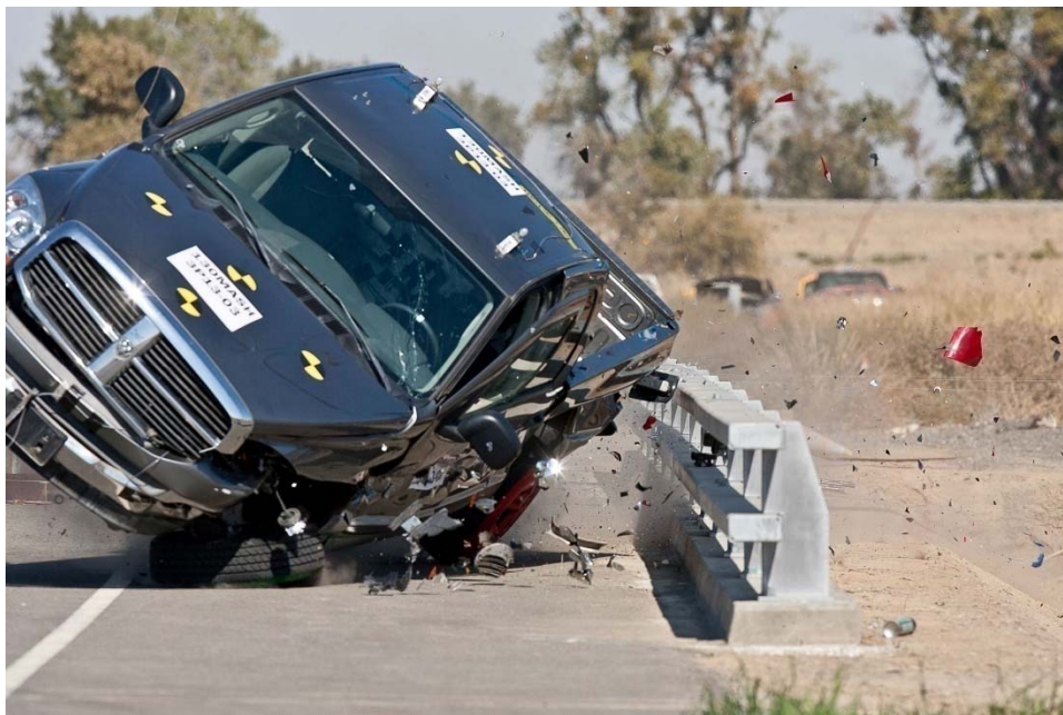
Figure 5-9 Vehicle Riding on Drive Side Front Tire
