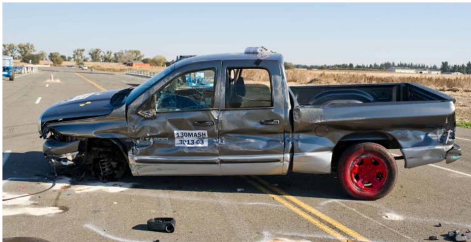
Figure 5-15 Side of Upright Vehicle After Test 130MASH3P13-03
