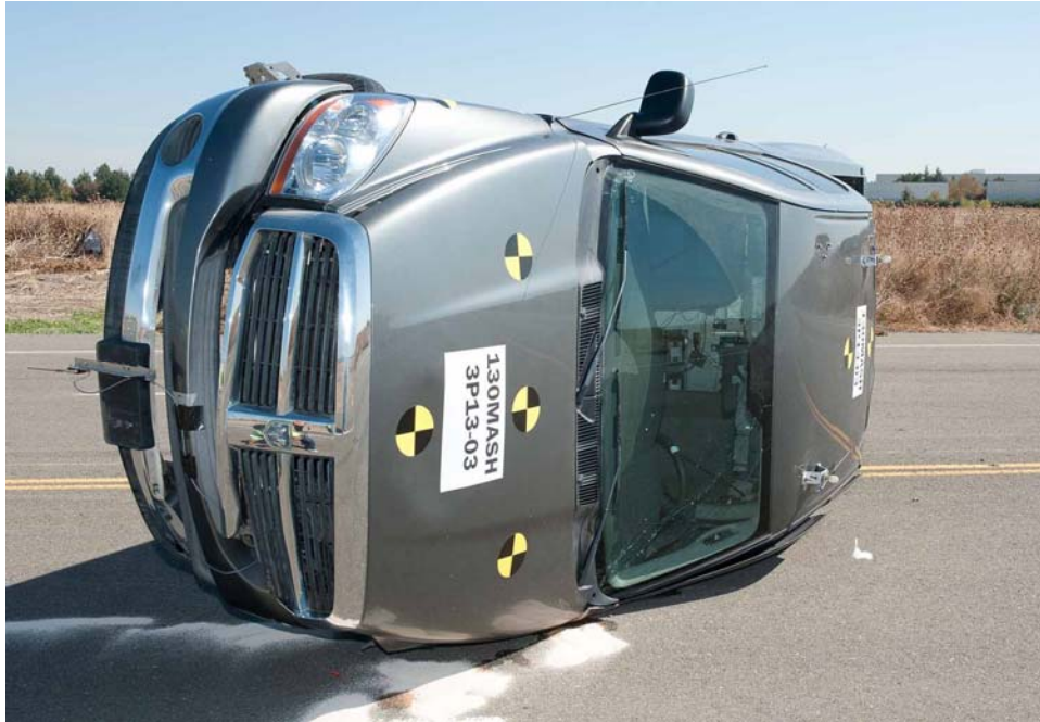
Figure 5-10 Front of Vehicle on Its Side After Test 130MASH3P13-03
