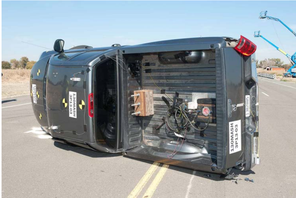
Figure 5-12 Back of Vehicle on Its Side After Test 130MASH3P13-03
