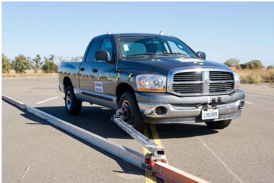
Figure 4-1 Test Vehicle Guidance System
