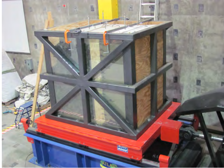
Figure 7. Shake table test of MSE wall
