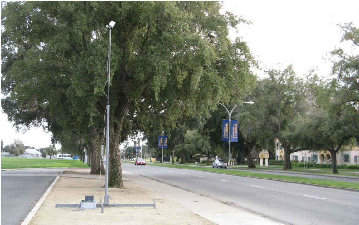
Figure 8: RTMS Mast for Rapid Deployment (View Looking South, Nov 12, 2010)
