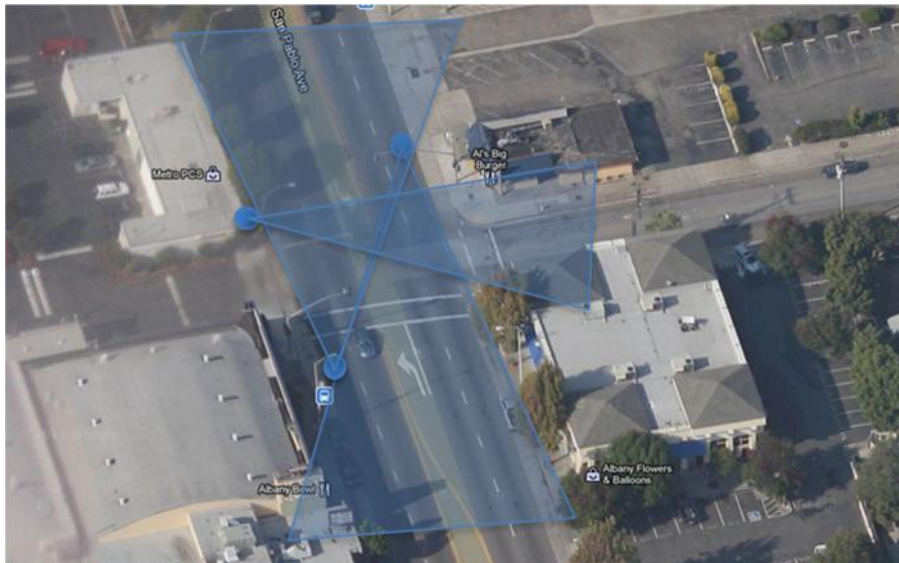
Figure 7.5 Placement of Radar Sensors: San Pablo Avenue and Brighton Avenue, Albany, CA
