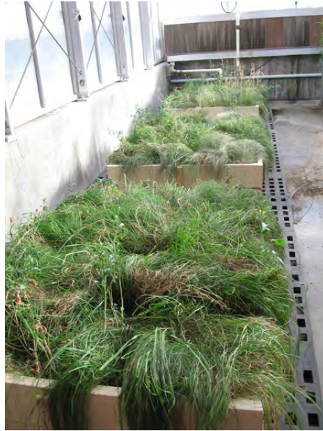
Figure 3.6 Three deep soil boxes each with 12 transported sod pieces (both high and low initial planting density) on reinforcement mats or bare ground. Dried weeds can be seen breaking through the sod.
