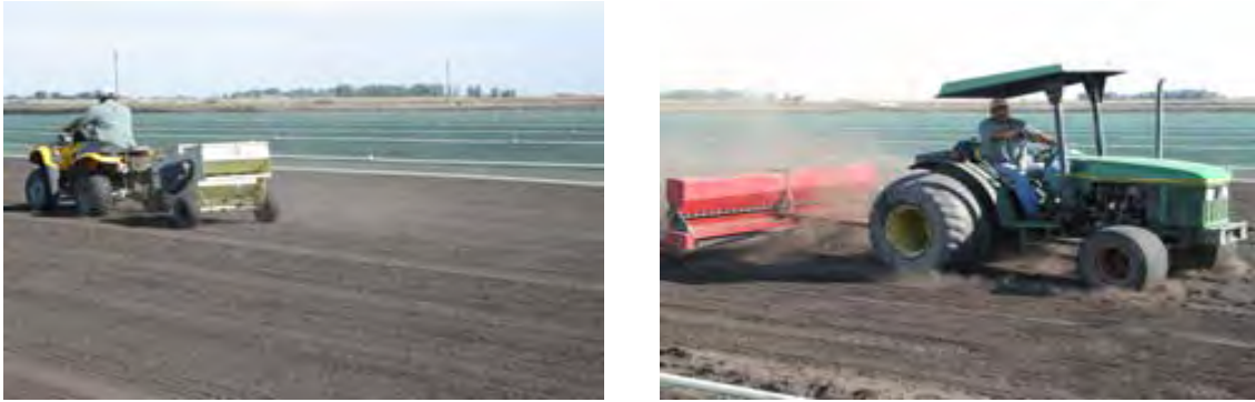
Figure 5.11 Grass seeder (left photo) and Brillion seeder used to pack and cover the seed (right photo) at the Delta Bluegrass Company farm in September 2007.
