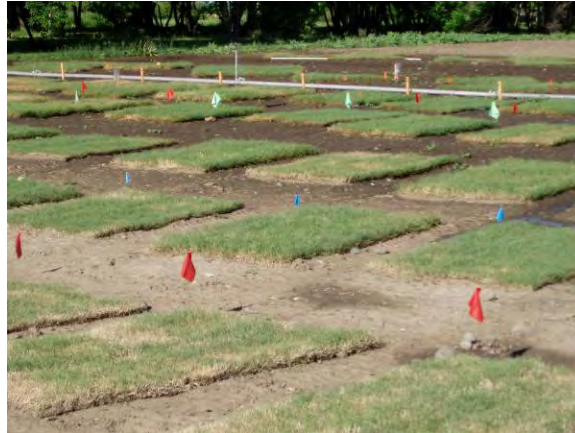
Figure 4.2 The line-source used to establish the four levels of irrigation regime plus a no irrigation control (Experiment A 1 ).
