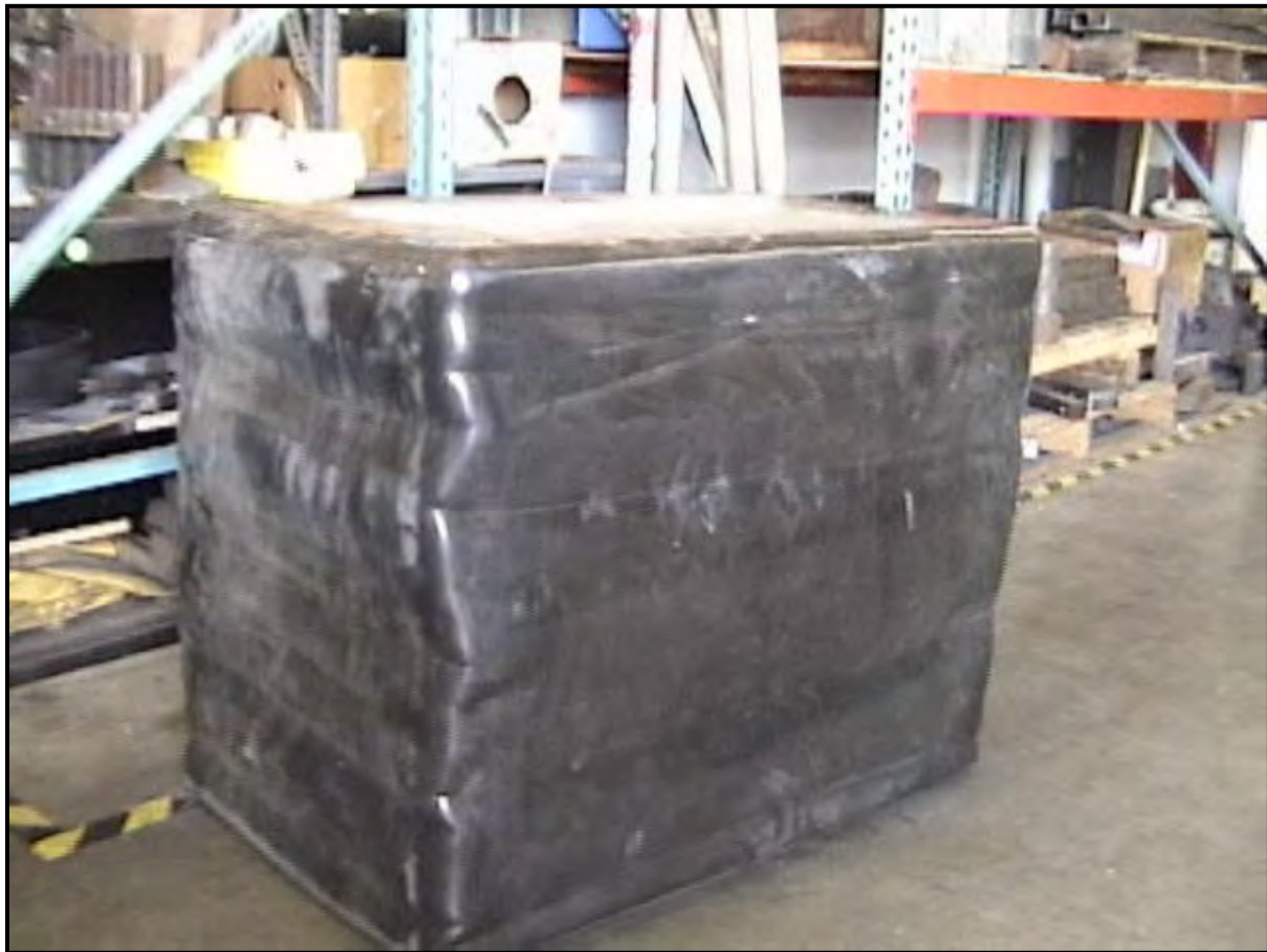
Figure 6-11 Test Sample 10 Minutes After Unloading 30" Dimension Now Almost 29"
