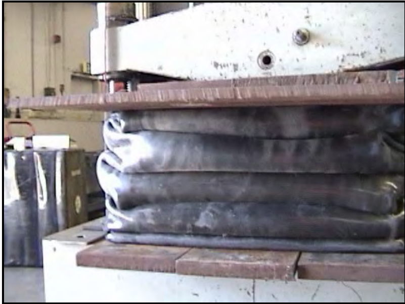
Figure 6-10 Fully Compressed Module, About 10" Deep
