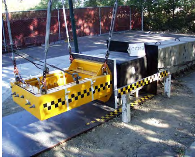
Figure 6-20 Test Set-Up, With Swing Mass at Nadir of Trajectory
