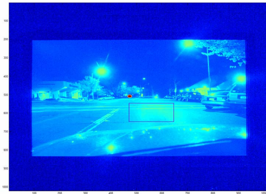
Figure 8a. This picture (previously seen in Figure 5) shows the area taken for background comprising matrix entries from row 550 to 650 (inclusive) and column 475 to 650 (inclusive). This area is shown bordered by a purple rectangle.
