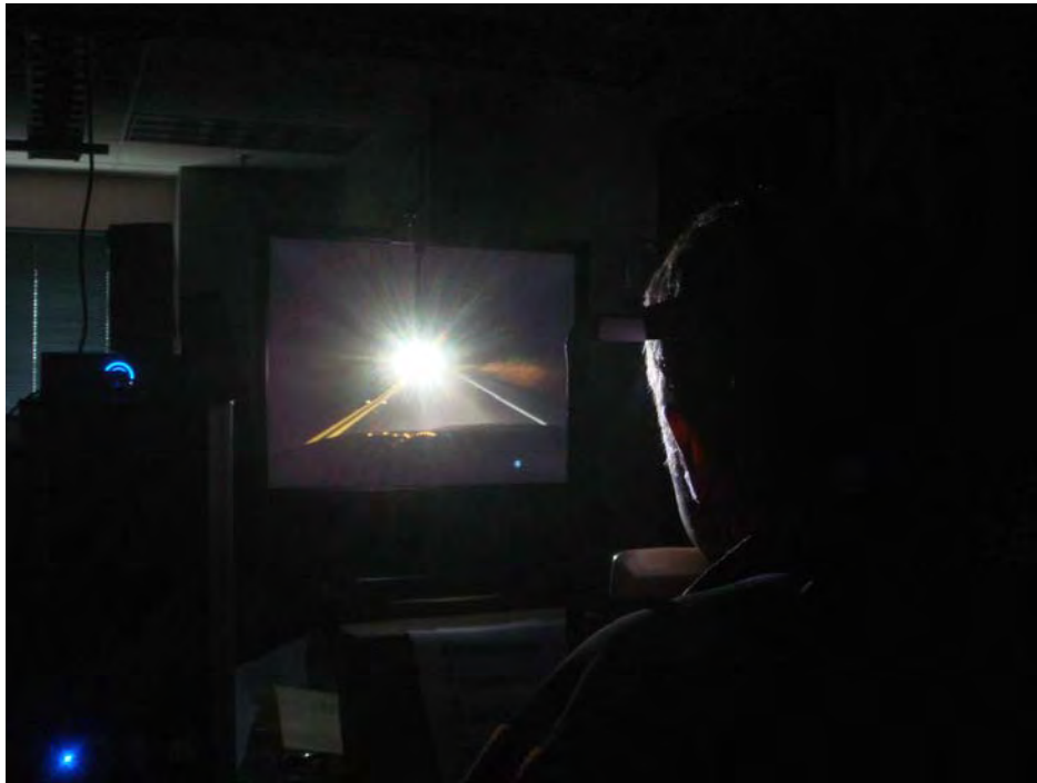
Figure 3c. Observer is viewing the rural scene where there is no roadway lighting. The glare source is at high intensity and in the position closest to the direction of gaze, simulating hi-beam headlights of an opposing vehicle.
