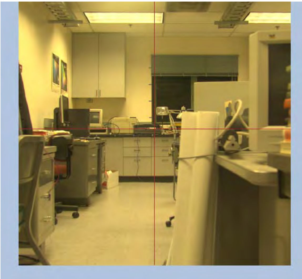
Figure 1. Entire “True Color” image (with superfluous blue border) for the 1020 x 1020 photometer array. The Nikon lens was used; it was focused at “infinity” and the f-number was f/8. The ProMetric software used “measurement #8”, that is ND2 for the three tristimulus values and exposure times of Y = 25 s, X = 100 s, and Z = 300 s along with “dark imaging”. The distance from the front surface of the lens to the front of the countertop was 21' 3". There was an additional length of 30.5" from the front of the countertop to the wall.
