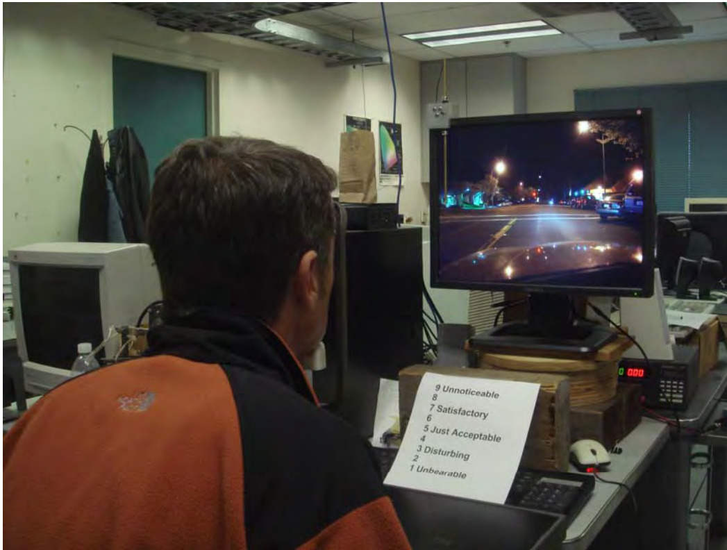
Figure 2. Experimental setup for the discomfort glare experiment. In the actual experiments the room was darkened and the glare source, which can be seen near the left edge of the display, was activated.
