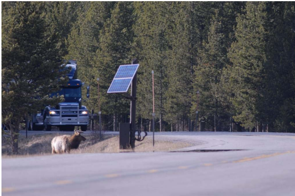
Figure 5.1: A bull elk (in velvet) approached the system on 25 April 2007, and activated the warning signs. The activated warning signs in combination with the high visibility of the elk next to the road resulted in vehicles braking and reducing speed (Personal observation Marcel Huijser, WTI-MSU) (Photo: Marcel Huijser, WTI-MSU).
