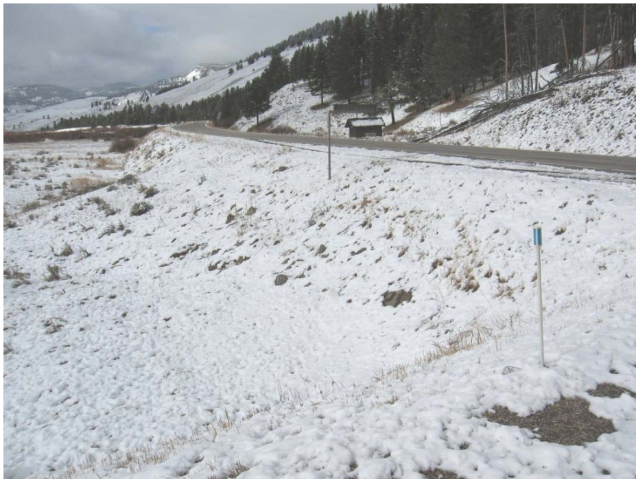
Figure 2.14: Looking north from the Black Butte Ranch access road towards Station 21. There is a blind spot in the area between the Black Butte access road and Station 21, because the sensor on Station 23 had to be placed high on the pole in order to shoot across the embankment of the Black Butte access road (see Figure 2.12) (Photo: Marcel Huijser, WTI-MSU).
