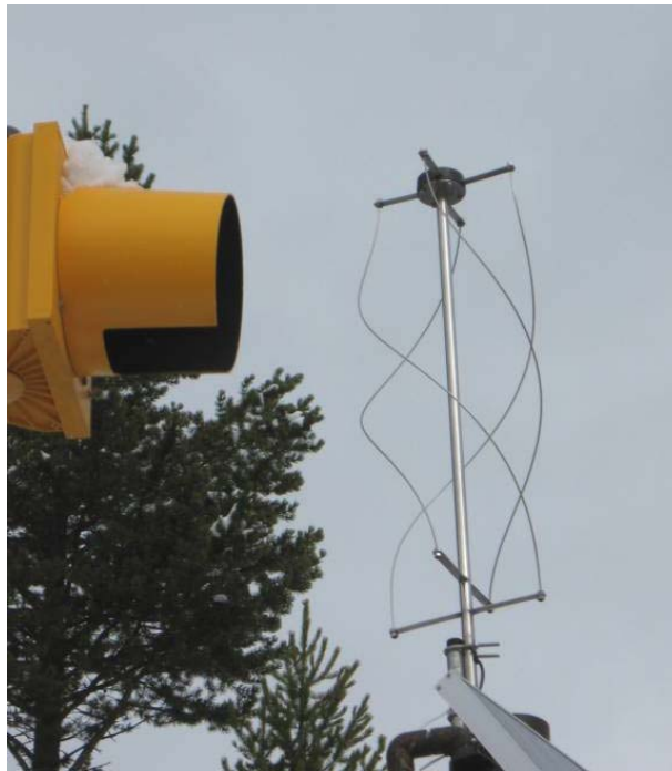
Figure 2.11: Antenna for remote access through satellite connection (Photo: Marcel Huijser, WTI-MSU)
