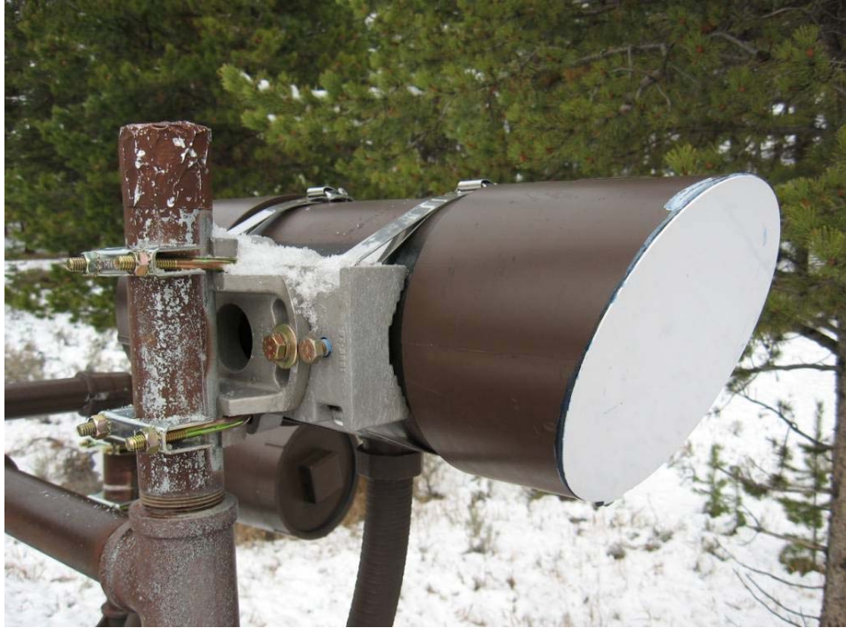
Figure 2.10: Sensor equipped with new bracket (aluminum casting, metal bands around sensor tube) (Photo: Marcel Huijser, WTI-MSU)
