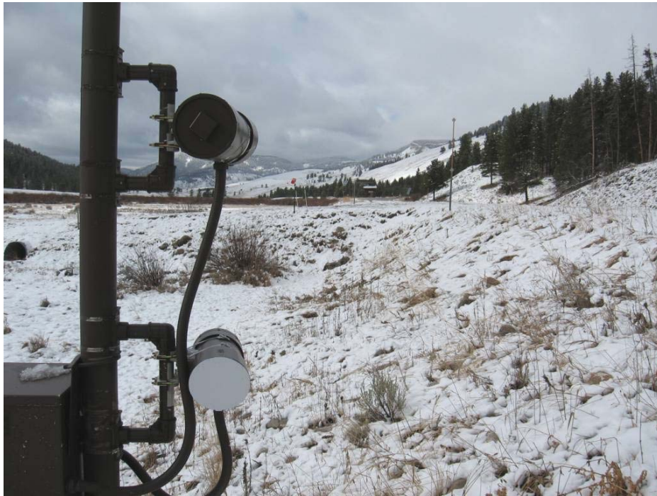
Figure 2.12: Looking north from Station 23 (Detection Zone 3) towards the Black Butte Ranch access road and Station 21. There is a blind spot in the area between Station 23 and the Black Butte access road because the sensor had to be placed high on the pole in order to shoot across the embankment of the Black Butte access road (Photo: Marcel Huijser, WTI-MSU).
