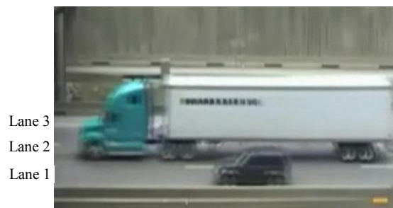
Figure 3.5, A video frame corresponding to the case where a pulse of a combined splashover bounds the pulse of the valid detection from lane 2. In this case, the difference of on-times is -6/60 seconds.
