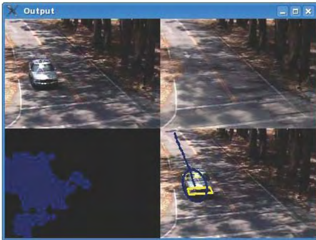
Figure 2.13. Vehicle tracking with virtual loop matched with real loop on the ground
