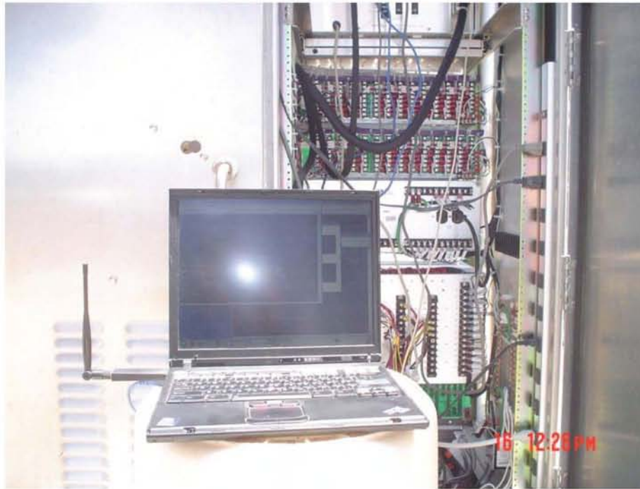
Figure 2.8. Laptop interfacing with C922 3M Canoga Card also runs IEEE802.11b wireless communication handshaking with the laptop computer running video camera
