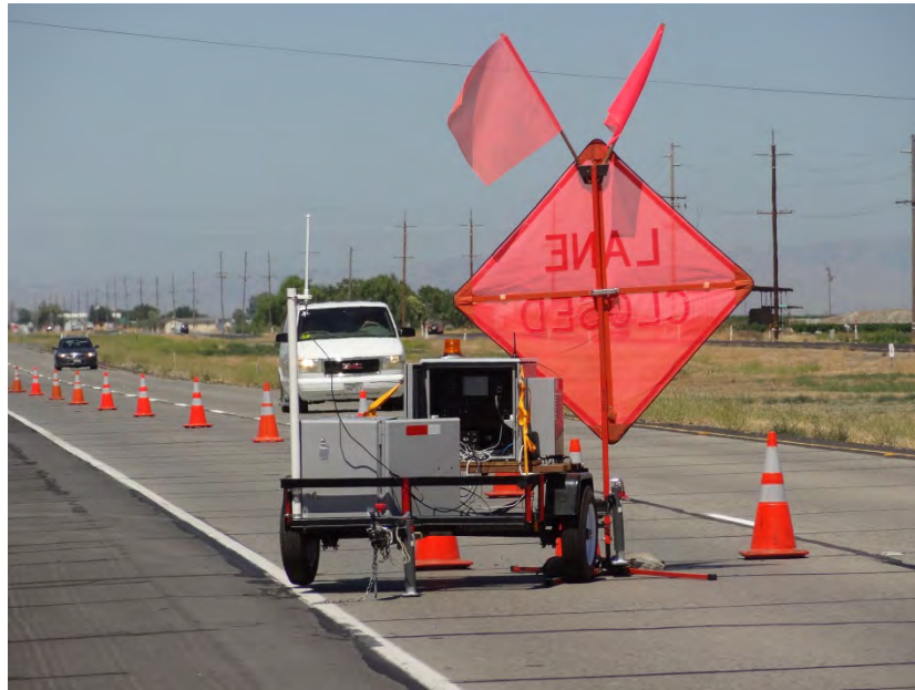
Figure 4. Placement of Speed Camera
