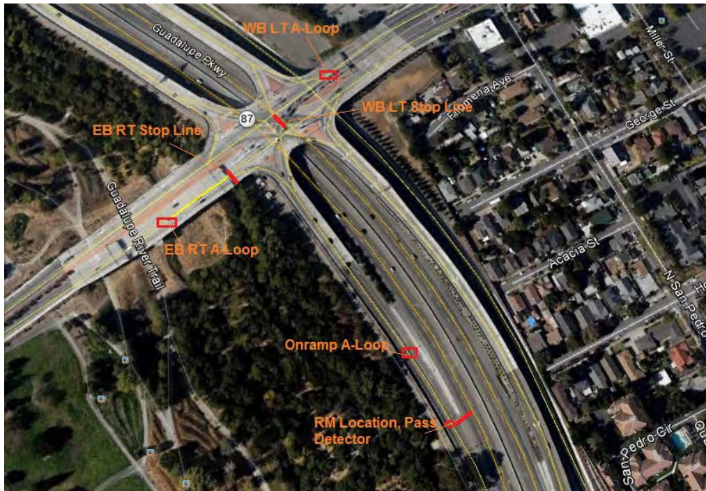
Figure 9-1. Relevant detector locations; distance of advance loops to the stop line: WB LT – 141[ft]; EB RT – 197 [ft].
