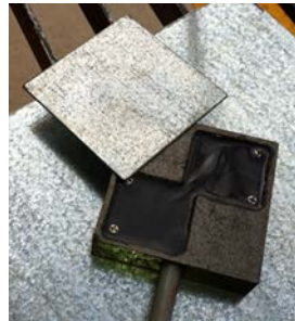
Figure 82: Magnetic accelerometer mount with cover.
