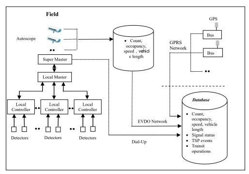
Figure 5-3: Data Collection System for VTA Line 22 Corridor
