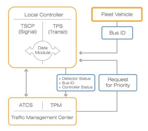
Figure 3-7: LADOT Centralized TSP System
