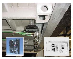
The AVI system as installed under a bus in Los Angeles County, California (Photo Credit: VTA, San Jose, CA)
