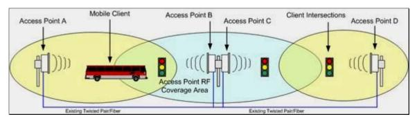
Figure 4-12: Typical WLAN Bridging Configurations
