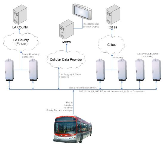
Figure 4-7: Signal Priority Communications Architecture
