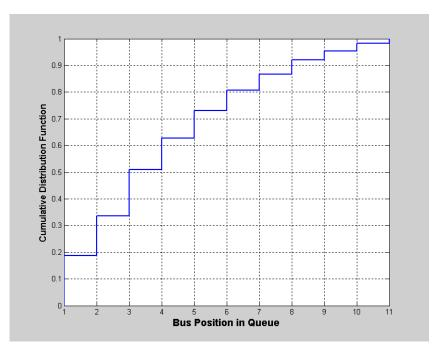
Figure 5-9 Empirical Cumulative Distribution Function of Bus Position in Queue
