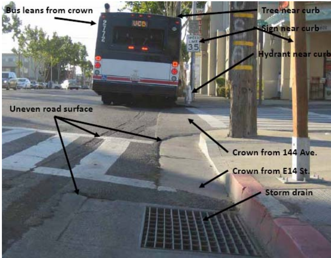
Figure 32 Station #2 Docking Precision Performance (Uneven Road Surfaces)
