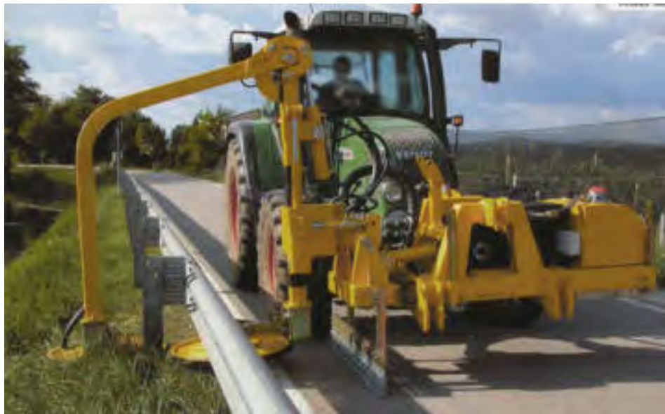
Figure 3.11 Tractor Mounted Guardrail Mower
