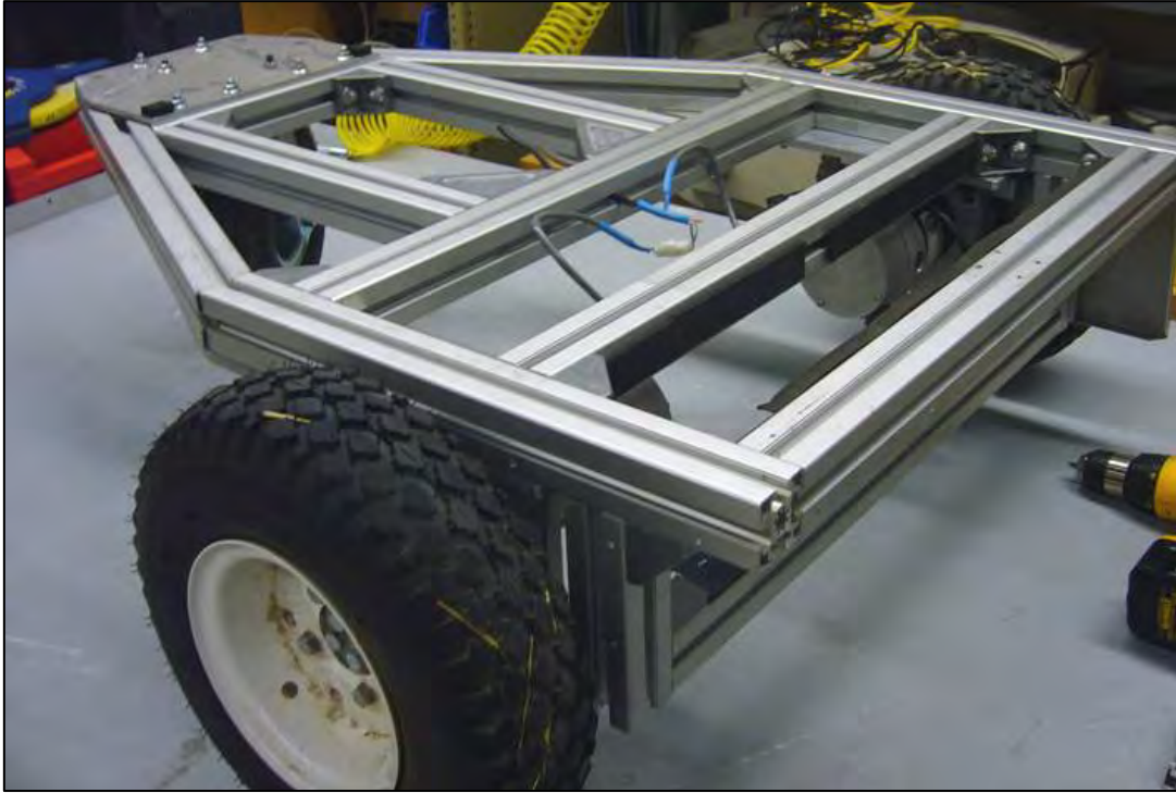
Figure 3.8 Testbed frame with mounted motors and wheels
