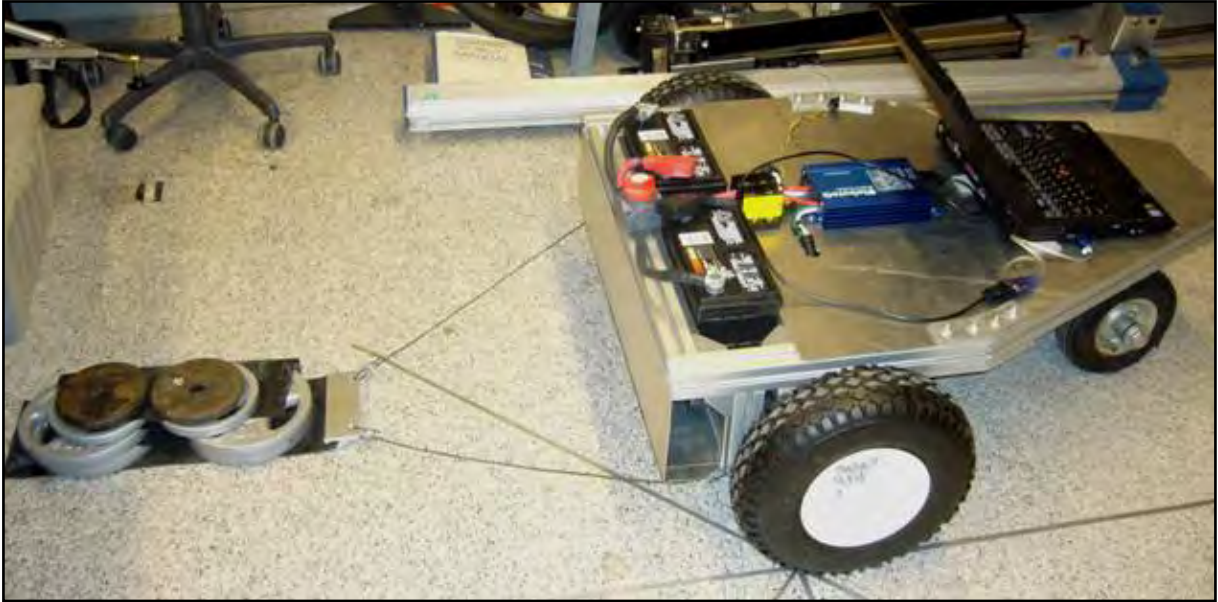
Figure A.10 PID tuning configuration with 60 lb (267 N) of weight pulled
