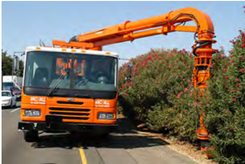
Figure 5.1 Advanced Roadway Debris Vacuum in Operation
