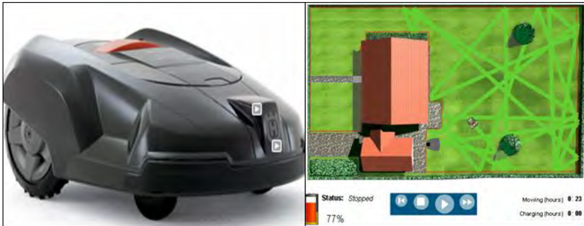
Figure 2.7 Automower (left), Simulated Random Cutting Pattern (right)
