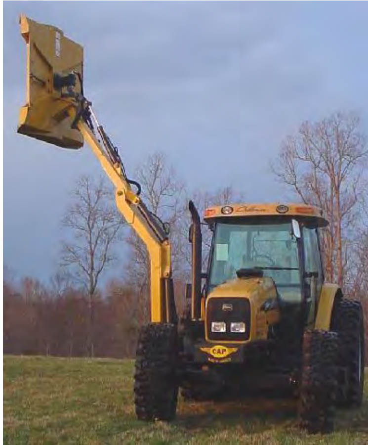
Figure 3.9 Tractor Mounted Boom Mower
