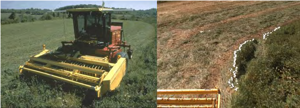
Figure 2.4 Automated Harvester (left), Sample output from crop line tracker (right) (From [28])
