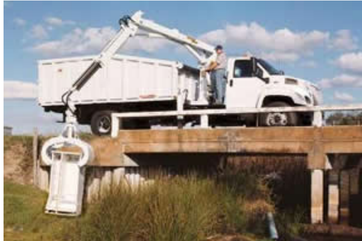
Figure 2-14 Grapple Truck Lifting Old Fridge
