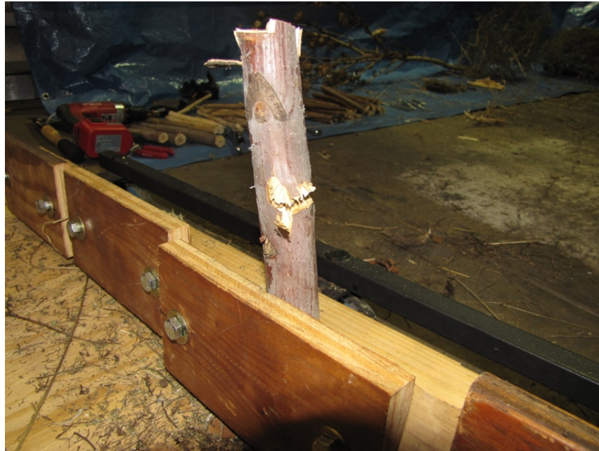
Figure 6-9 Failed Large Diameter Cut
