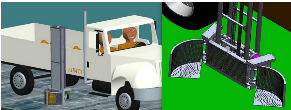
Figure 4-4 Debris Removal Attachment and Clamshell Action
