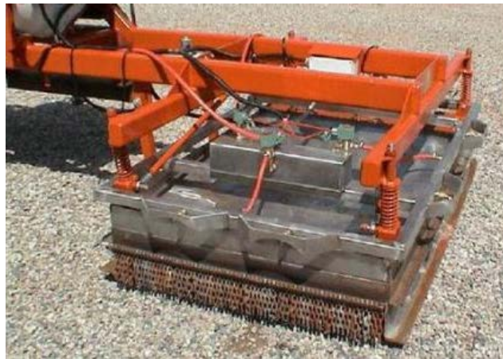
Figure 2-9 Radiant Heat Attachment
