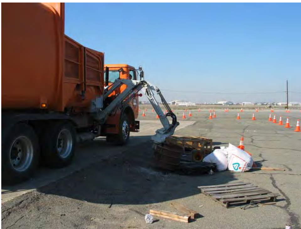
Figure 1.9: Latest revision of the Caltrans DRV is integrated with commercial arm
