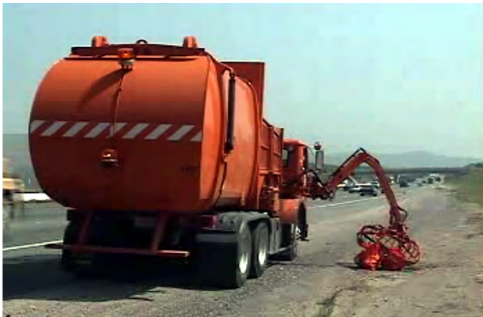
Figure 1.8: Dedicated Debris Removal Vehicle with Hydraulic Arm System [4]
