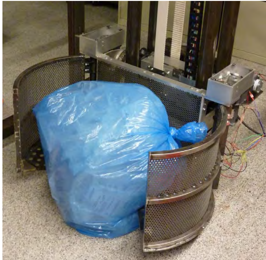
Figure 6.9: Clamshell Design Iteration #1
