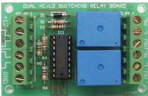
Figure 3.9: Two Channel Relay Board [18]
