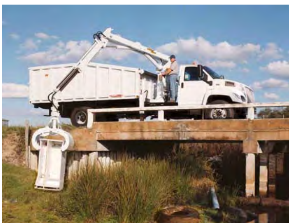
Figure 1.6: Large grappler system, (image from Wikipedia)
