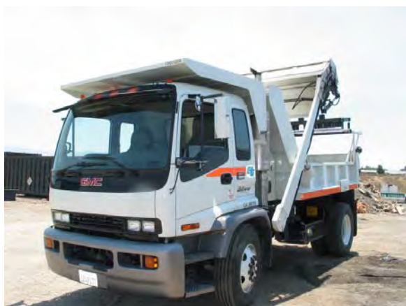
Figure 1.4: Caltrans dump body with loader
