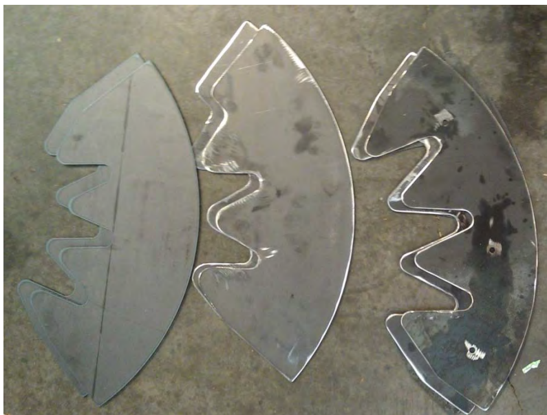
Figure 6.12: Multiple Tooth Plates before installation
