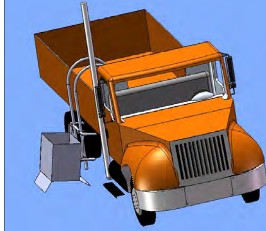
Figure 2.4: Horizontal jaws and a track which allows for vertical and rotational movement.
