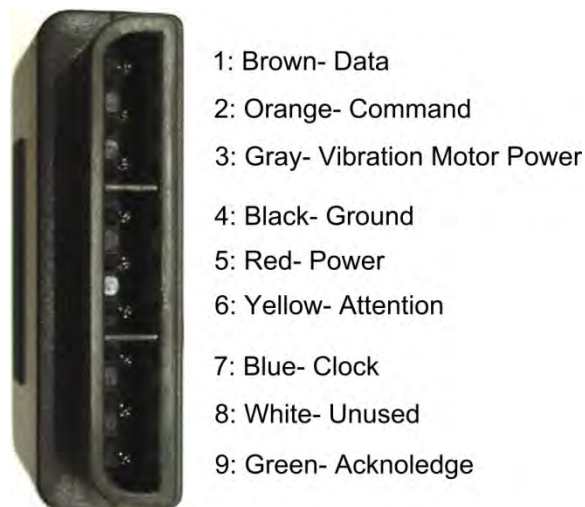
Figure 5.1: PlayStation 2 Wire Colors and Uses [32]
