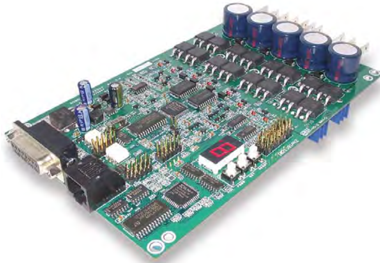
Figure 3.6: AX3500 High Power Motor Controller by RoboteQ [13]
