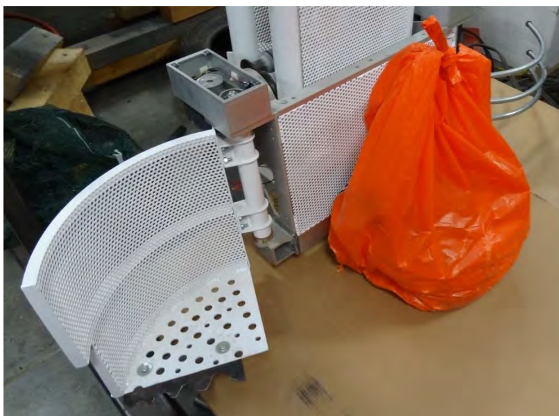
Figure 6.11: Configuration used for scooping bags of debris
