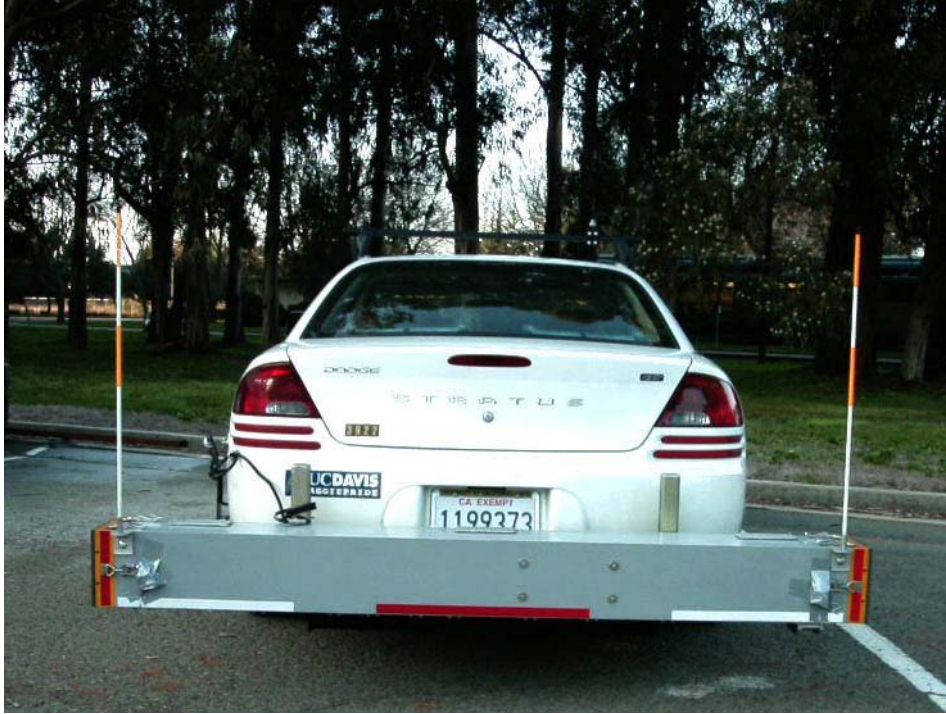
Figure 22: Laser profilometer beam.
