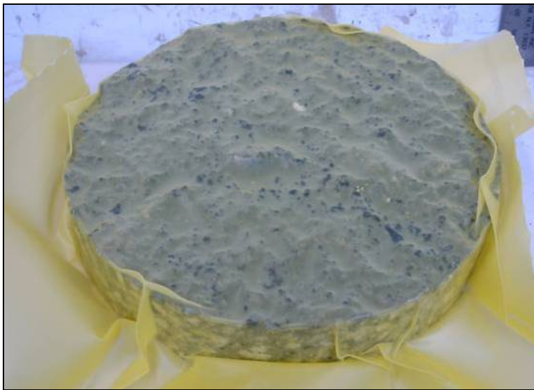
Figure 24: CoreLok seal of specimen.
