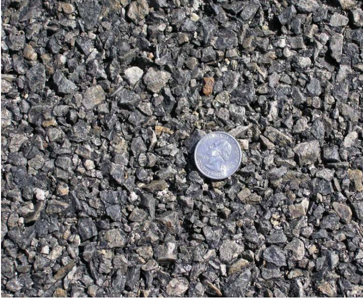
Figure 13: Rubberized open-graded asphalt concrete (RAC-O).
