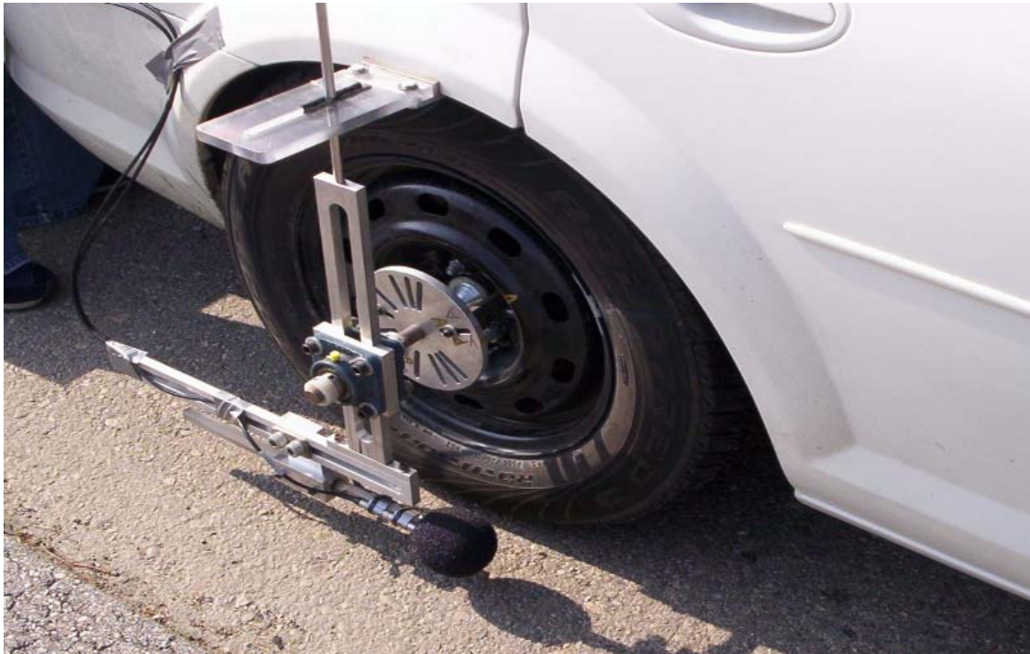
Figure 21: On-board sound intensity (OBSI) microphone setup.
