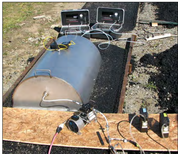
Figure 3.1: Portable flux chamber schematic and field sampling setup.
