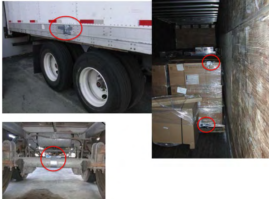
Figure 3.23: Company B accelerometer detail.
