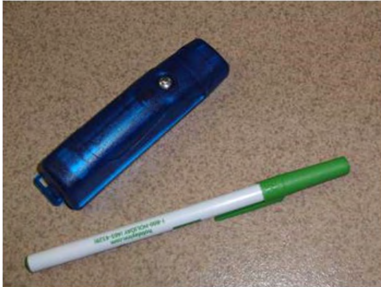
Figure 3.1: Accelerometer used for collecting acceleration data from trucks and freight.
