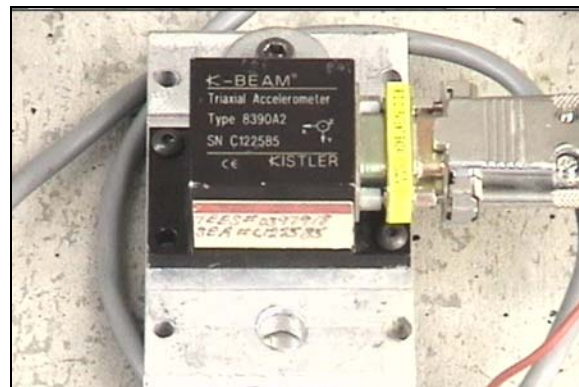
Figure 7.11. Accelerometer Attached to Watson Wash Bridge Structure
