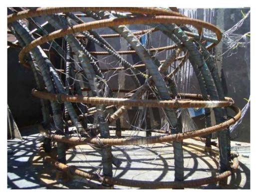
Figure 3.85: Close up of bottom of Specimen I after collapse
