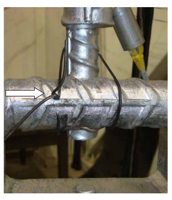
Figure 3.15: Fracture of Single-U Tie Wire Connection
