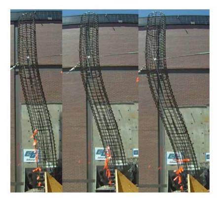
Figure 3.71: Sequence of deformed shapes for Specimen I, view from West
