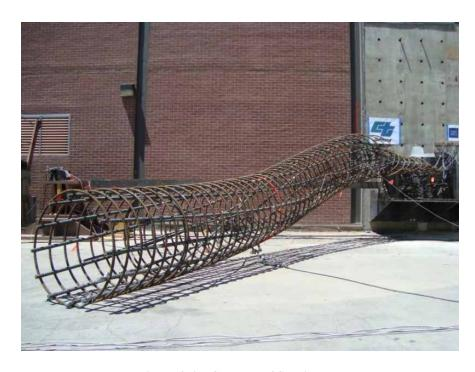
Figure 3.67: Collapse of Specimen I
