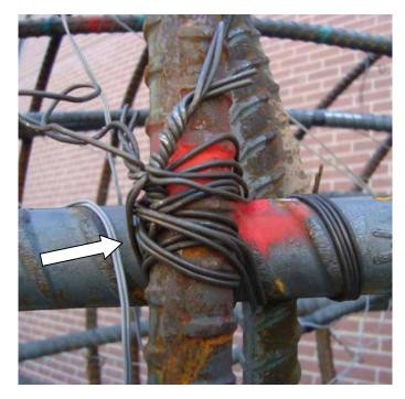
Figure 3.73: Strong-tie intact after rebar cage collapse
