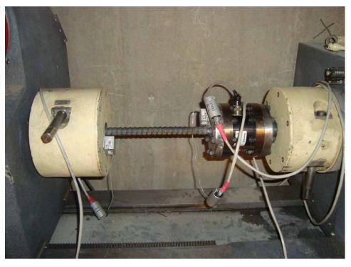
Figure 3.40: Test Set-up for Torsion of a rebar
