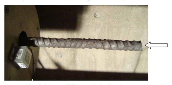
Figure 3.42: Fracture of #6 Bar under Torsional Loading
