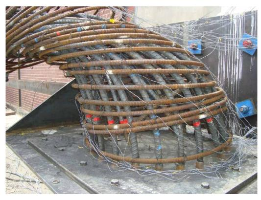
Figure 3.100: Close up of Specimen II bottom after collapse
