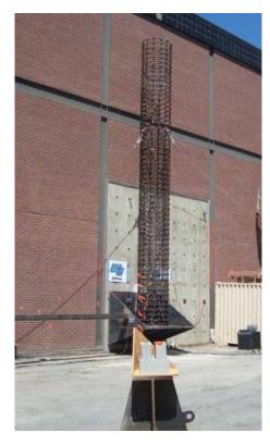
Figure 3.50: Specimen I standing without any Temporary Support
