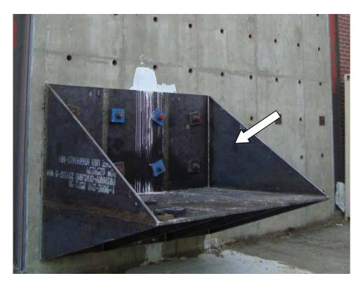
Figure 3.54: Details of Steel Bracket Attachment
