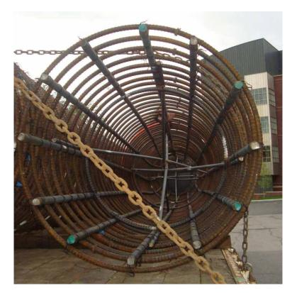
Figure 3.47: X-braces of Specimen I
