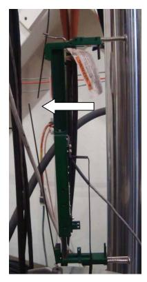
Figure 3.3: Failure of Tie Wire Coupon
