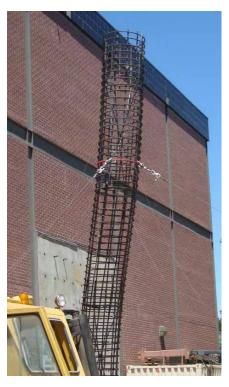
Figure 3.69: Specimen I deformed shape, view from South-West
