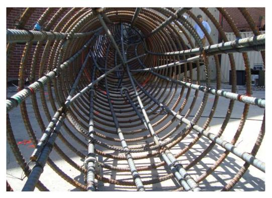
Figure 3.84: Top Brace after collapse of Specimen I
