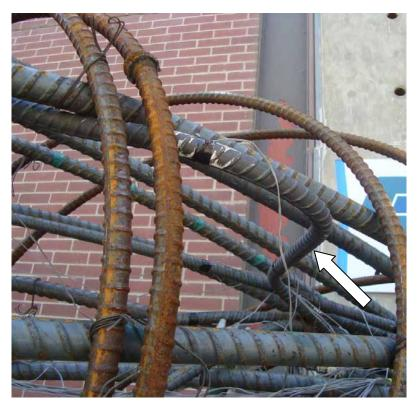
Figure 3.82: Close up of buckled brace bar after collapse of Specimen I
