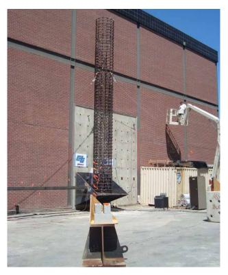
Figure 3.59: Specimen I Test Set-Up
