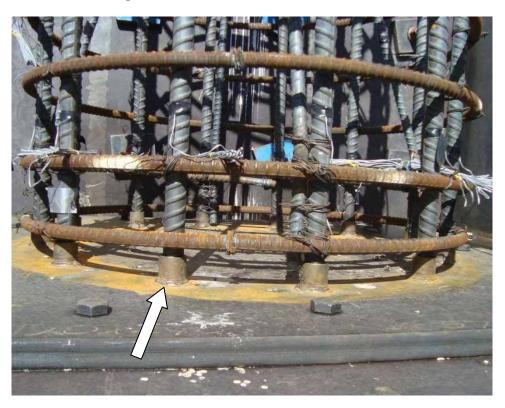
Figure 3.55: Base of the Rebar Cage with the Longitudinal Bars Welded to the Base Plate
