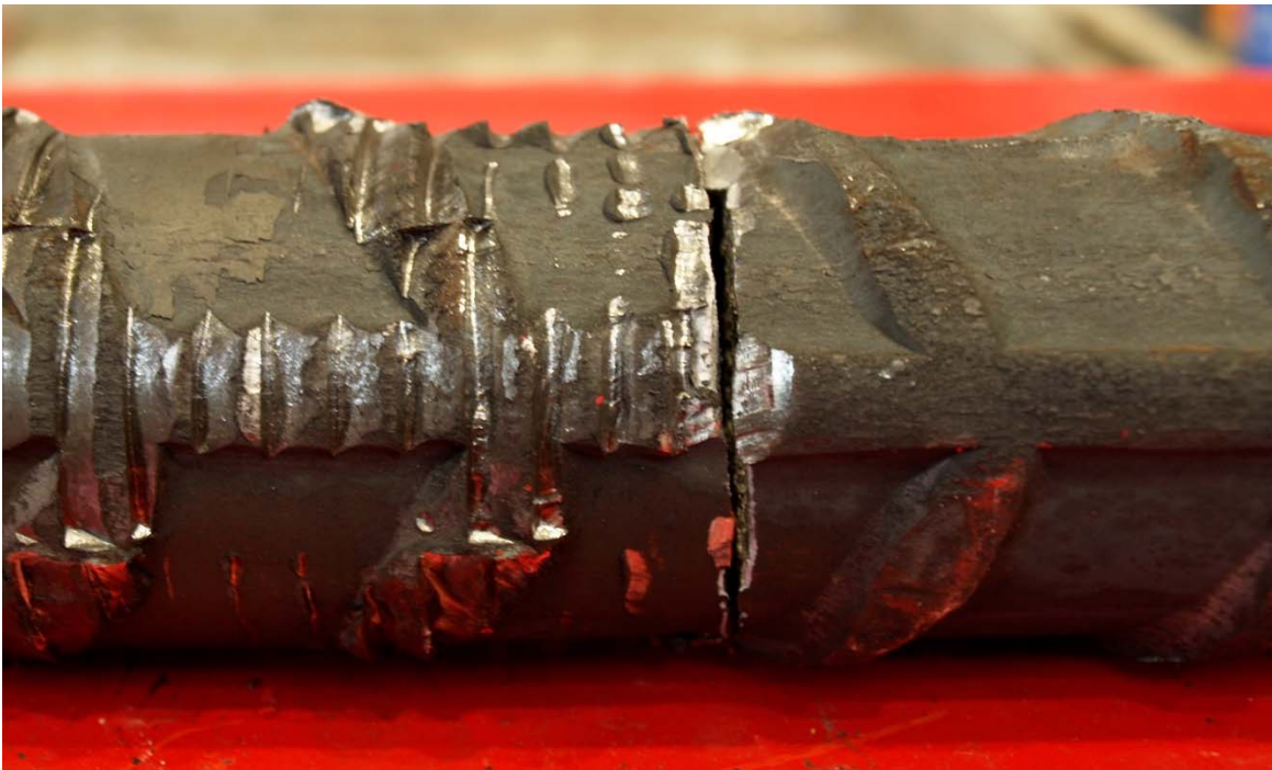
No. 18 Bar – brittle failure at grips early into necking
