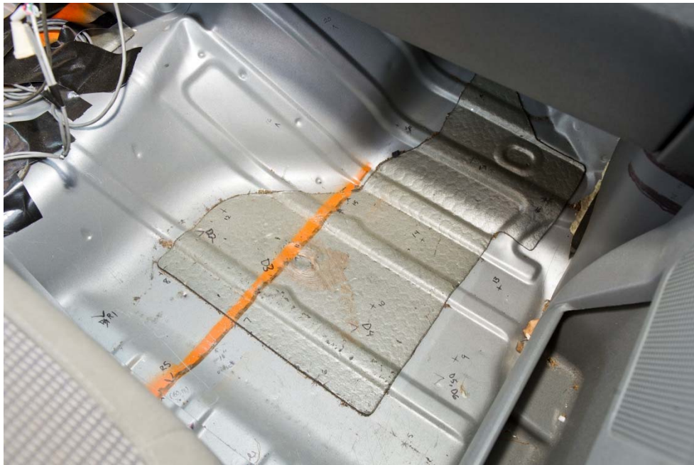
Figure 3-8 – Floorboard deformation of test vehicle after Test 130MASH3P13-01
