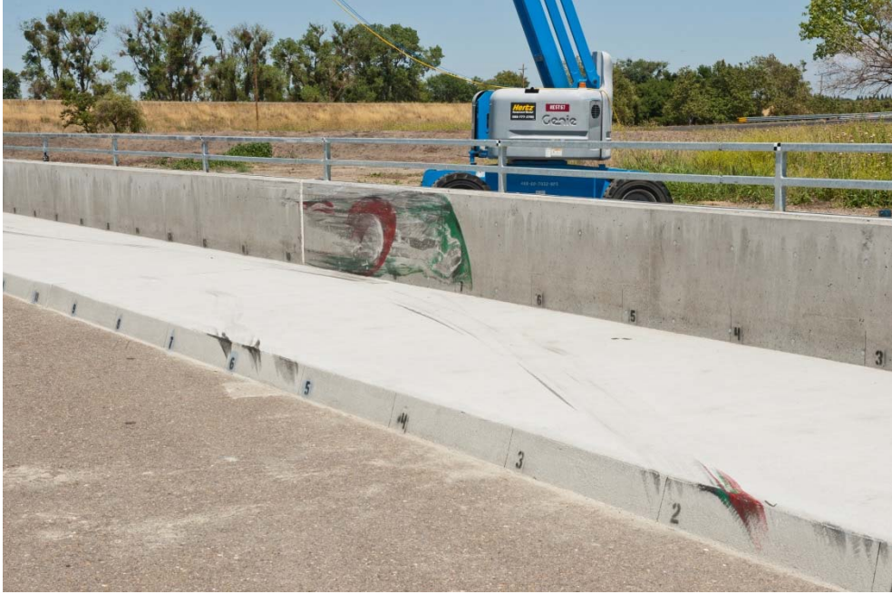
Figure 3-2 – Type 732SW Barrier after Test 130MASH3P13-01
