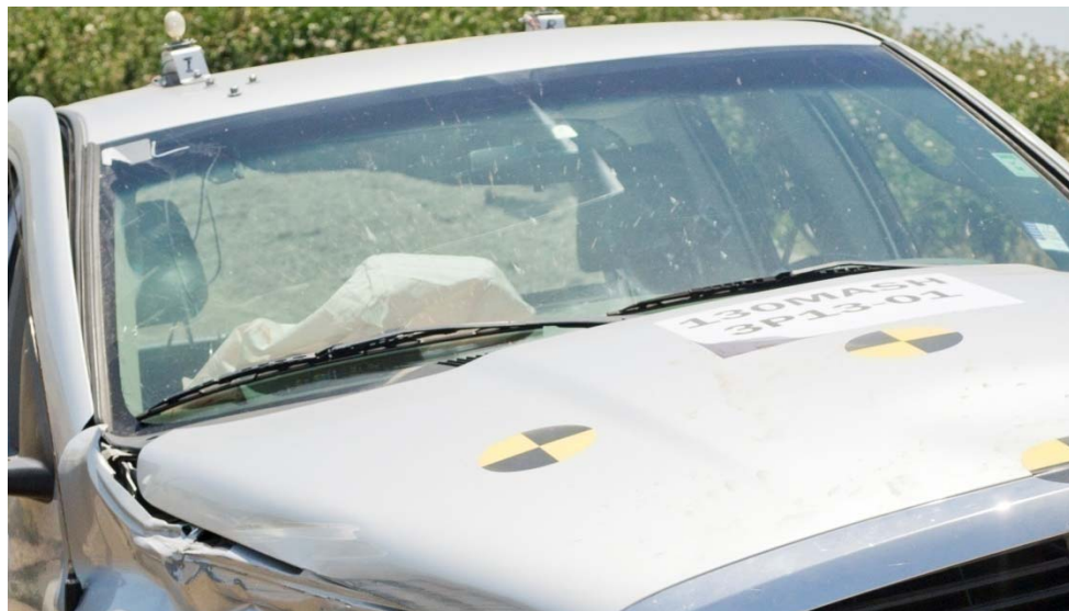
Figure 3-10 – Vehicle windshield after Test 130MASH3P13-01
