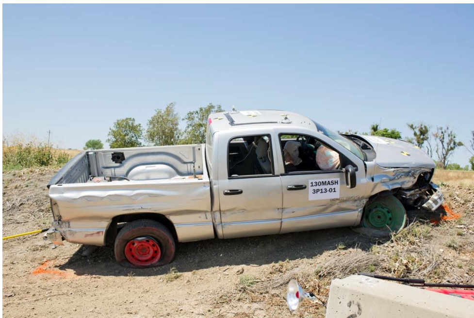
Figure 3-6 – Test vehicle after Test 130MASH3P13-01
