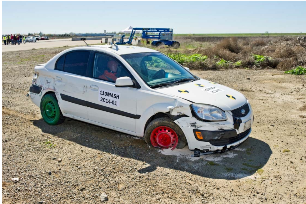
Figure 3-29 – Front right corner of test vehicle after Test 110MASH2C14-01
