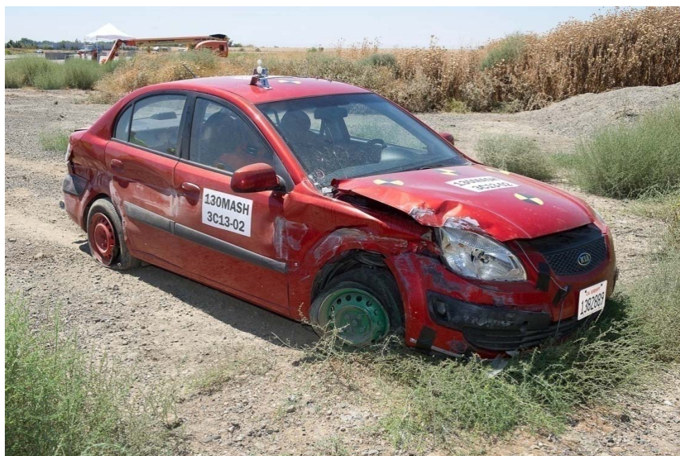
Figure 3-18 – Front right corner of test vehicle after 130MASH3C13-02
