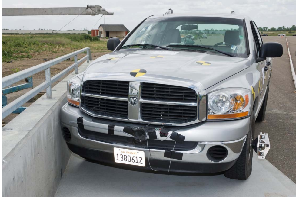
Figure 3-5 – Impact Condition for Test 130MASH3P13-01
