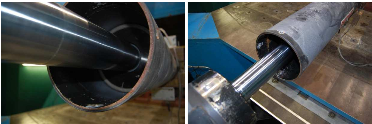
Figure 14. (a) inside view of the dry sleeve cover and clean front bearing for SN#003 damper, (b) inside view of the oily sleeve cover for SN#006 damper indicating mild leakage at front bearing.
