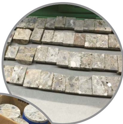
Pavement and bridge cores after cutting for visual inspection
