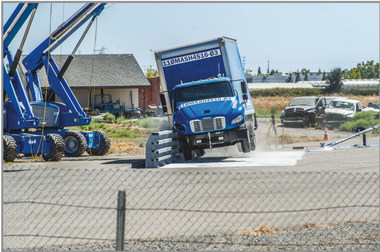
Testing the Caltrans-designed ST-70SM side-mounted bridge rail to verify that it meets the MASH criteria as a Test Level 4 longitudinal barrier. It successfully contained and redirected all three levels of vehicles and impact conditions as required.
