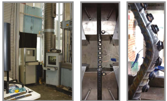
Buckled bar tension test (left); rebar with optical markers (center); buckled rebar (right)
