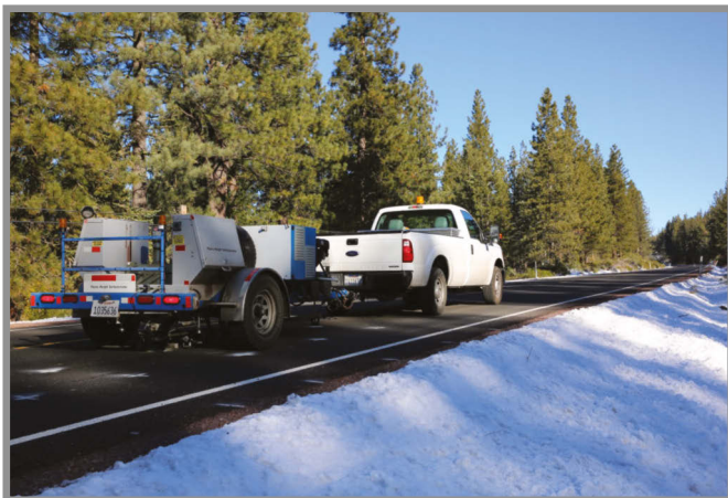
Testing to assess stiffness change over time
