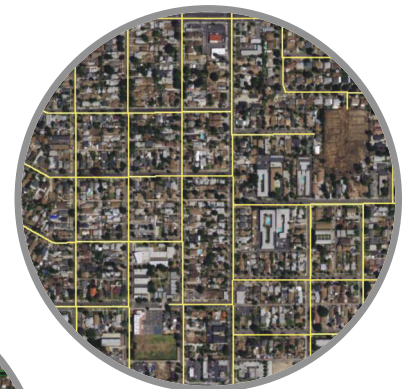
Outputs from initial digital processing of aerial images of the roadway network to create predictions of sidewalk locations. Yellow links are roadways, green links and blue nodes are sidewalks. Further image processing will validate the presence or absence of an actual sidewalk.
