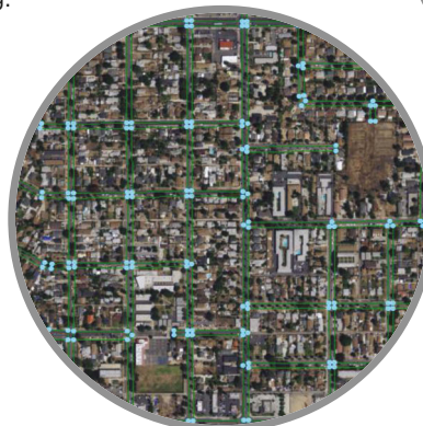
Outputs from initial digital processing of aerial images of the roadway network to create predictions of sidewalk locations. Yellow links are roadways, green links and blue nodes are sidewalks. Further image processing will validate the presence or absence of an actual sidewalk.
