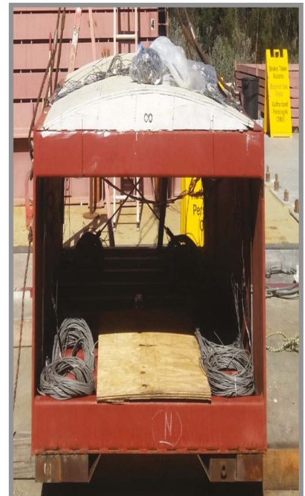
Large-scale shake table test model: model of tunnel structure
