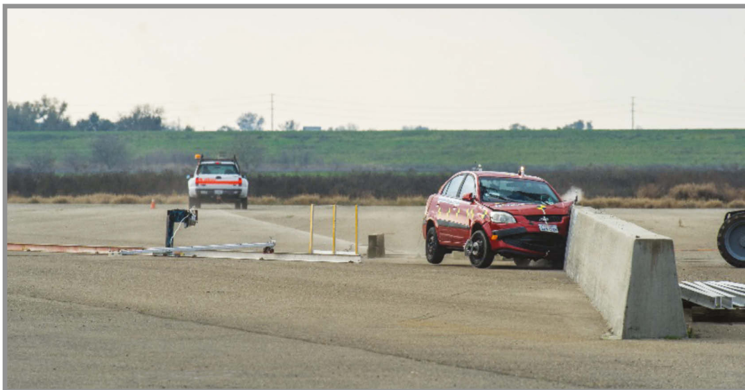
The Kia Rio sedan test vehicle was towed into the Type 60 barrier using a cable attached to a one-ton pickup. The researchers documented the test using still cameras, video cameras, high-definition high-speed digital video cameras, and data acquisition systems to record accelerations and rotational rate changes.
