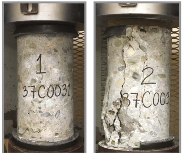
(Left) Bridge core in lab. (Right) Bridge core after testing.
