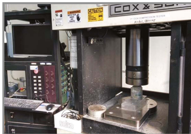
Pavement core strength testing
