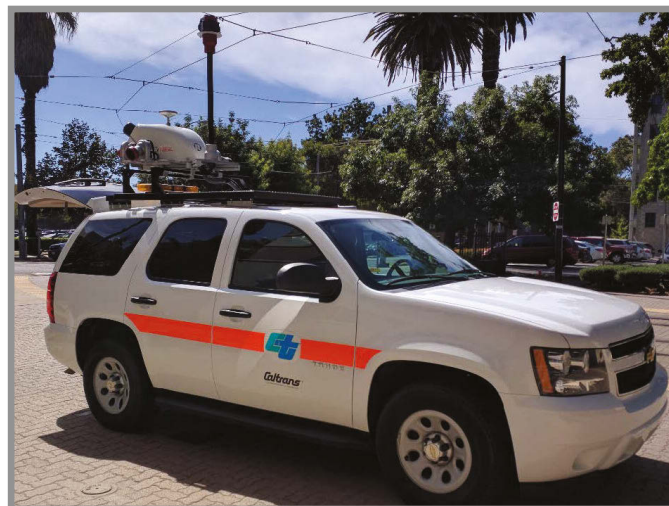
Riegl VMX-1HA sensor pod mounted on a custom roof rack
