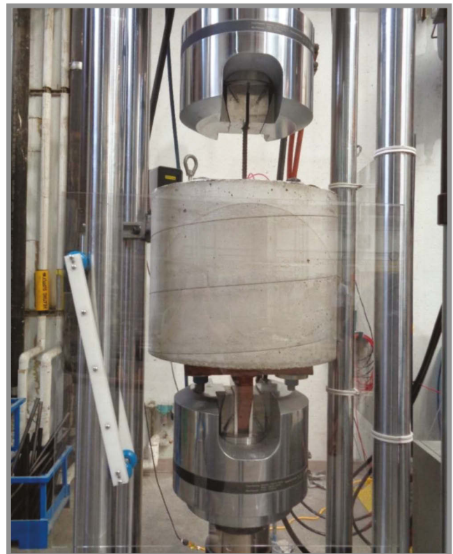
Pullout test setup
