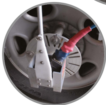
Distance measuring instrument mounted on the vehicle wheel
