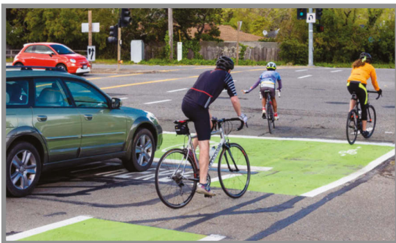
Bike boxes improve connectivity for bicyclists and pedestrians when crossing a major boulevard.
