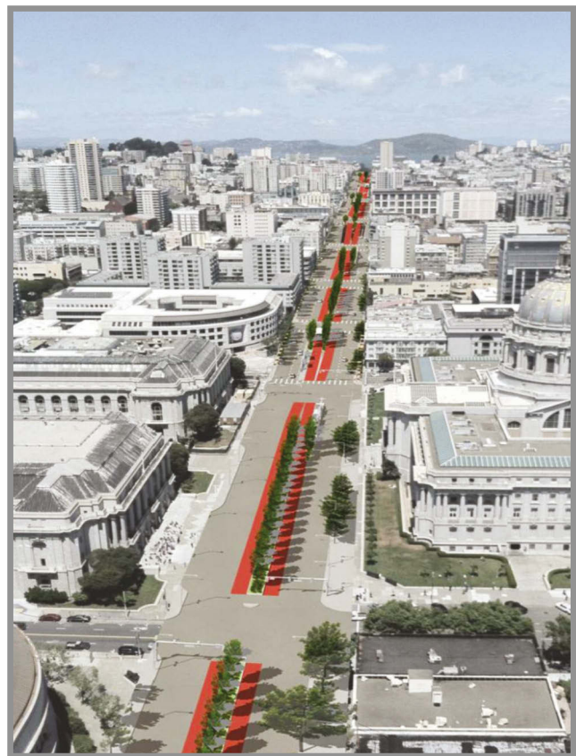
Rendering of Van Ness Avenue in San Francisco, with dedicated BRT lanes marked in red. The innermost lanes in each direction were historically subject to frequent delays as cars waited to complete left turns. Prohibiting left turns and adding BRT is projected to increase vehicle throughput per lane.
