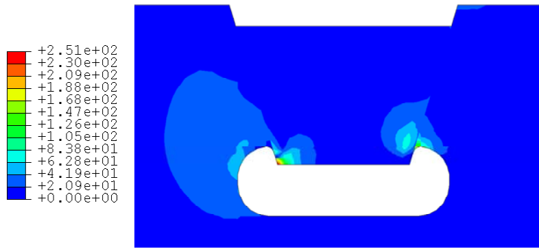
(a) Maximum Principal Stress on South Side (in Tension)
