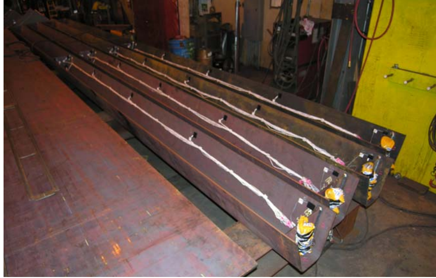
Figure 2.48 Strain Gage Instrumentation Inside of Ribs
