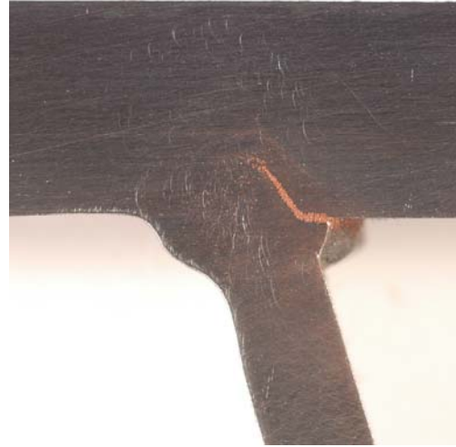
(b) Crack from Weld Root
