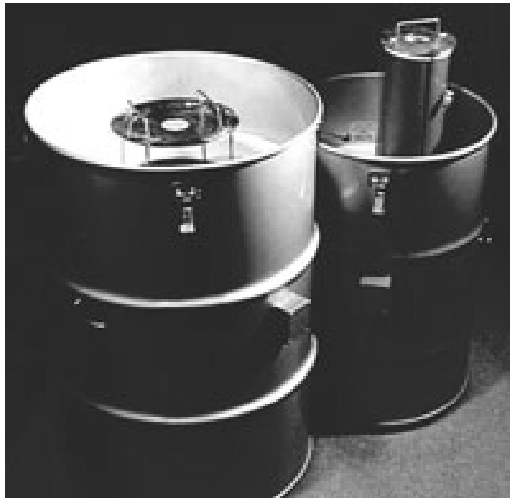
Figure B-1 – Q-Drum calorimeter
