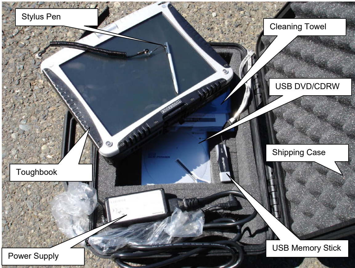
Figure 19 – Field borehole logging hardware
