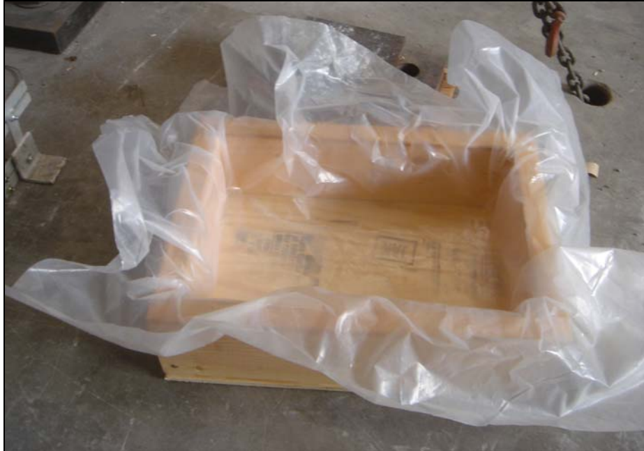
Figure 3.6: Sand-Jack with liner in place.
