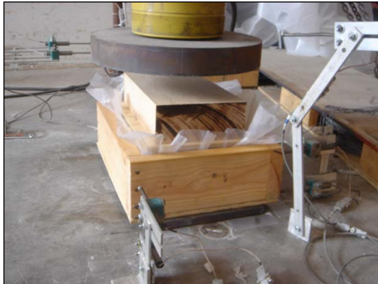
Figure 3.3: Sand-Jack with no banding and a plastic liner with hardwood spacer in place under load applicator.
