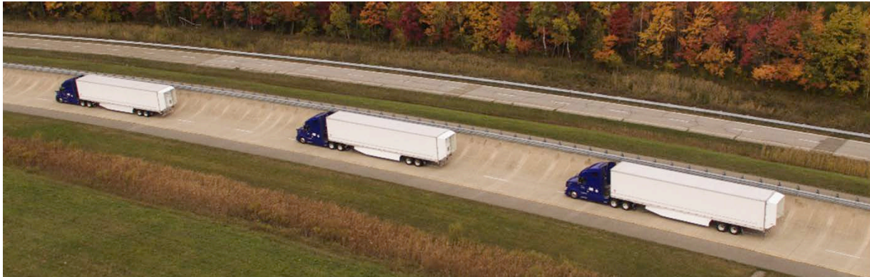
Figure 4–Truck CACC System Driven on Test Track at 65 mph, 0.6 second time gap (57 foot clearance gap)
