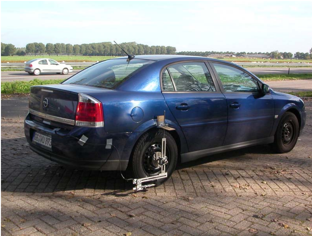
Figure 7: Photograph of the sound intensity measurement fixture installed on the Opel Vectra test vehicle in Europe
