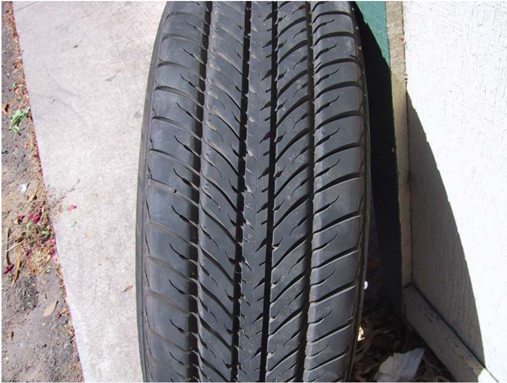
Figure 3a: Photograph of test tire tread patterns - Goodyear Aquatred 3 P205/70R15
