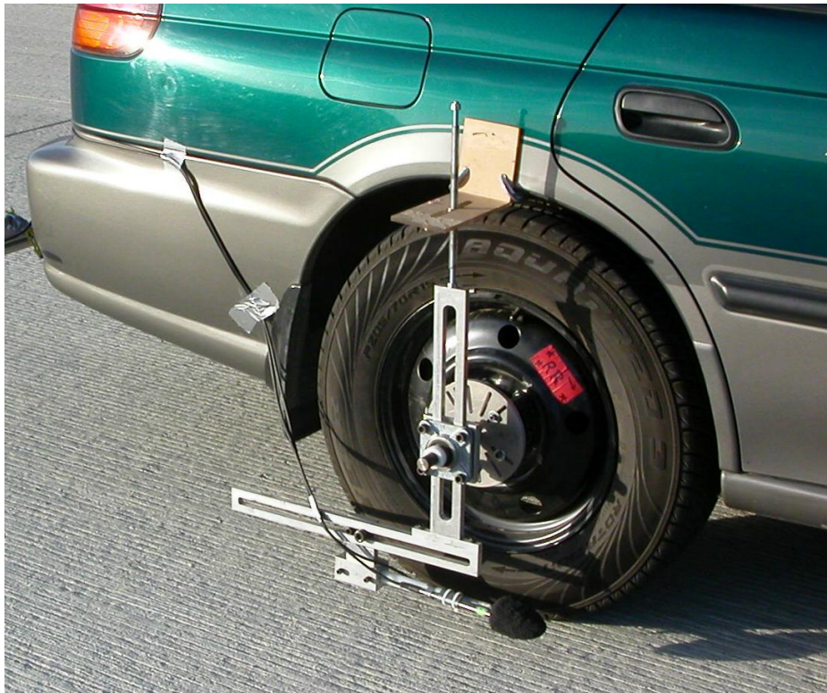
Figure 2: Photograph of the sound intensity measurement fixture installed on the right rear wheel of the test vehicle
