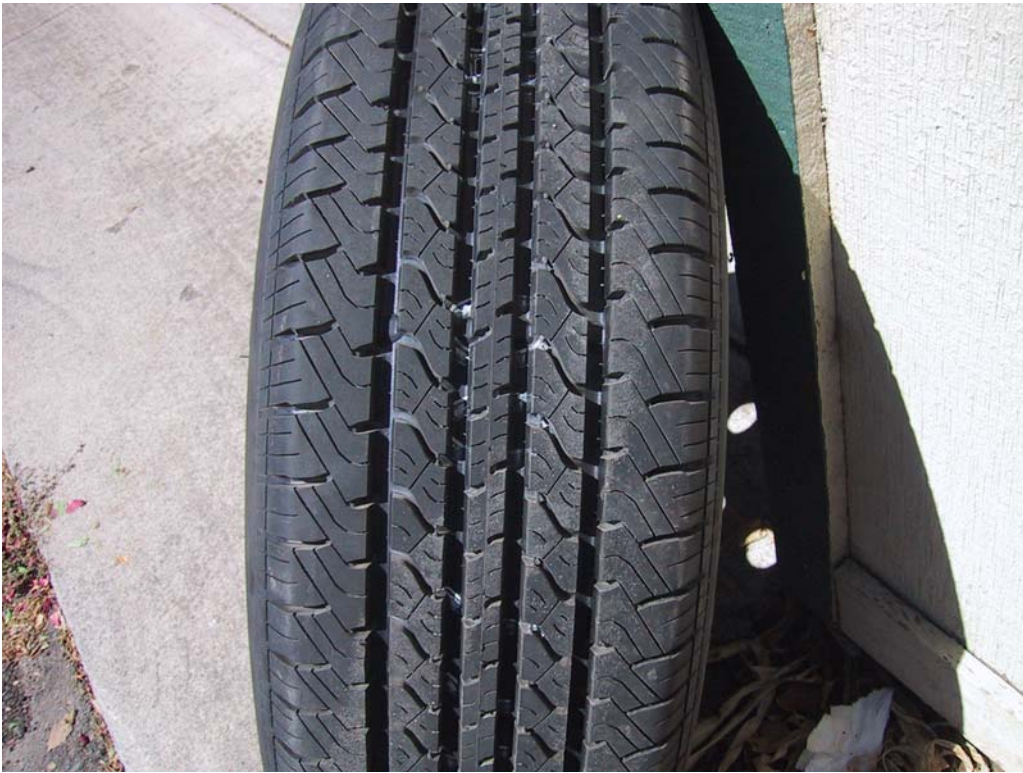
Figure 3a: Photograph of test tire tread patterns - Goodyear Aquatred 3 P205/70R15
