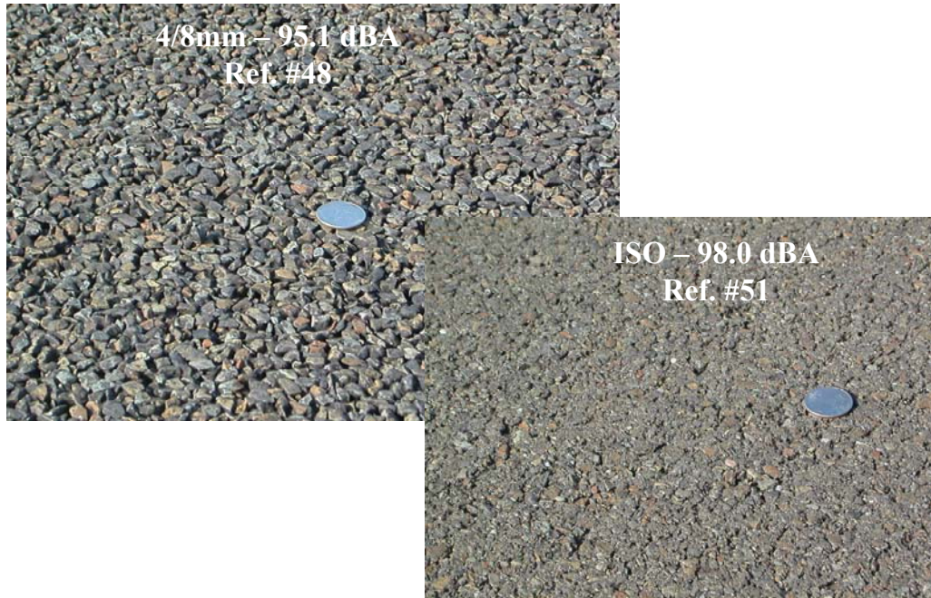
Figure 21: Photographs of two PA surfaces containing larger scale (a.) and finer scale (b.) aggregate and apparent surface roughness
