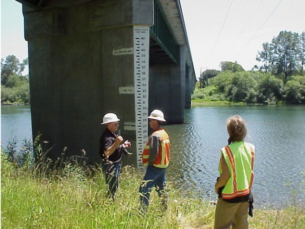
Smith River Stage Gaging Station at Dr. Fine Bridge
