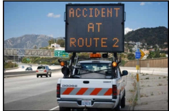
Incident Warning on Truck-Mounted PCMS
