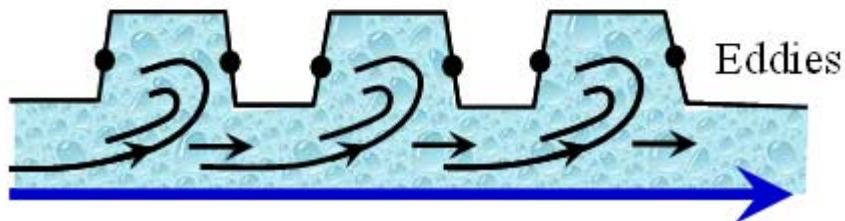
Figure 9-16. Hydraulic forces on cofferdams
