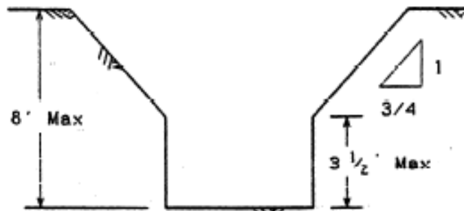
Unsupported Vertically Sided Lower Portion
